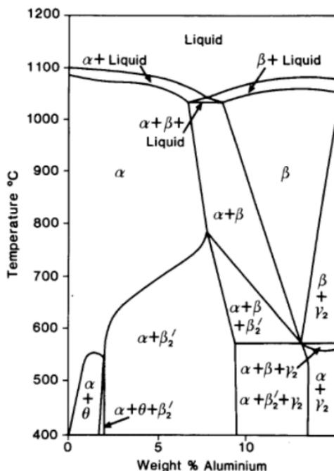
Figure 3: Vertical section of Cu-Al-Ni system at 3wt
