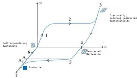
Figure 1: Schematic representation of the memory effect
