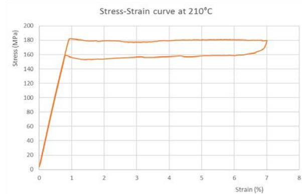
Figure 2: Tensile tests of Cu-Al-Ni single crystal samples at room temperature (martensitic state) (a) and at 210°C (austenitic state) (b)
