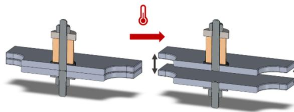
Figure 4: concept of a Murphy actuator for the dismantlement of a structure
