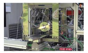
(b) Combustor during hot firing
