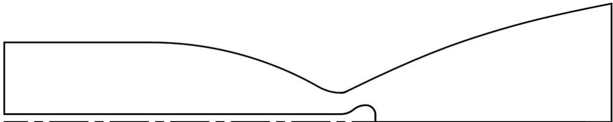
Figure 4: Basic reference ED nozzle (Case 1).
