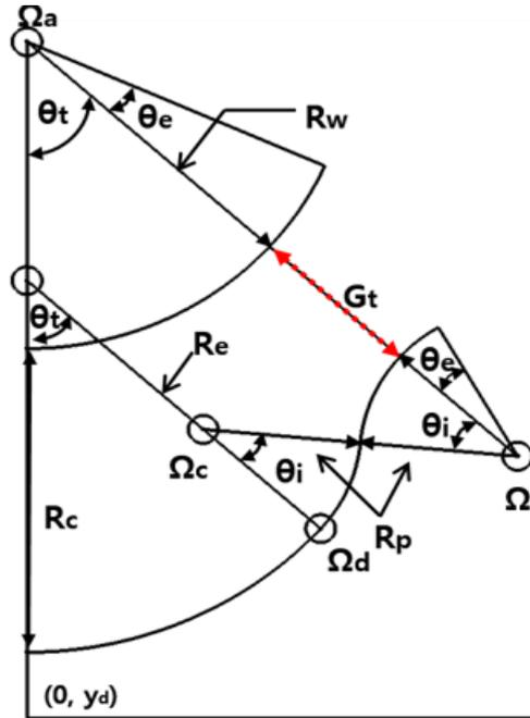
Figure 3: Schematics of E-D nozzle throat modelling method[9].
