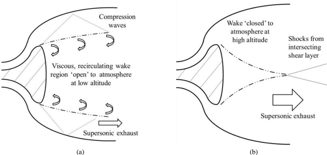
Figure 1: Flow Field in the ED nozzle (a) and open mode and (b) closed mode[2].
