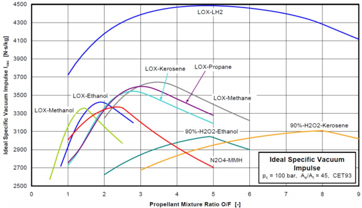
Figure 2: Performance of various propellant [47].
