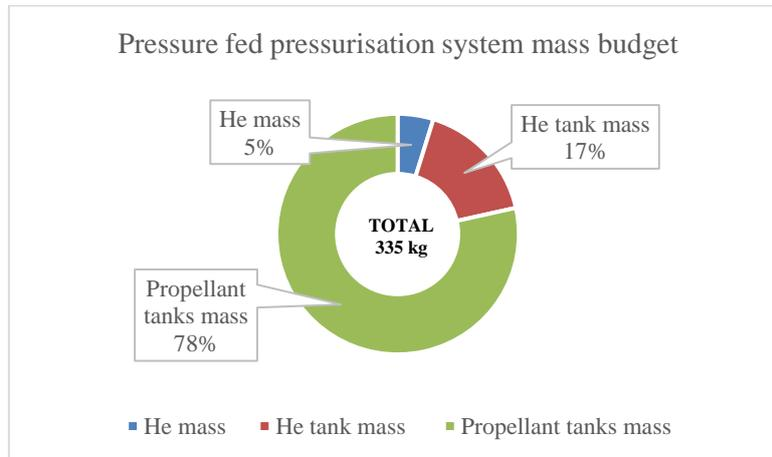
Figure 6: Pressure fed system mass distribution
