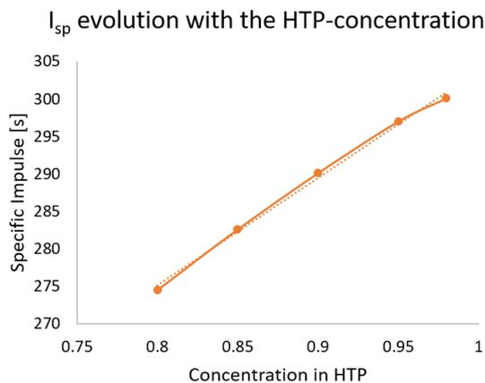
Figure 5: Evolution of the specific impulse with the concentration in hydrogen peroxide
