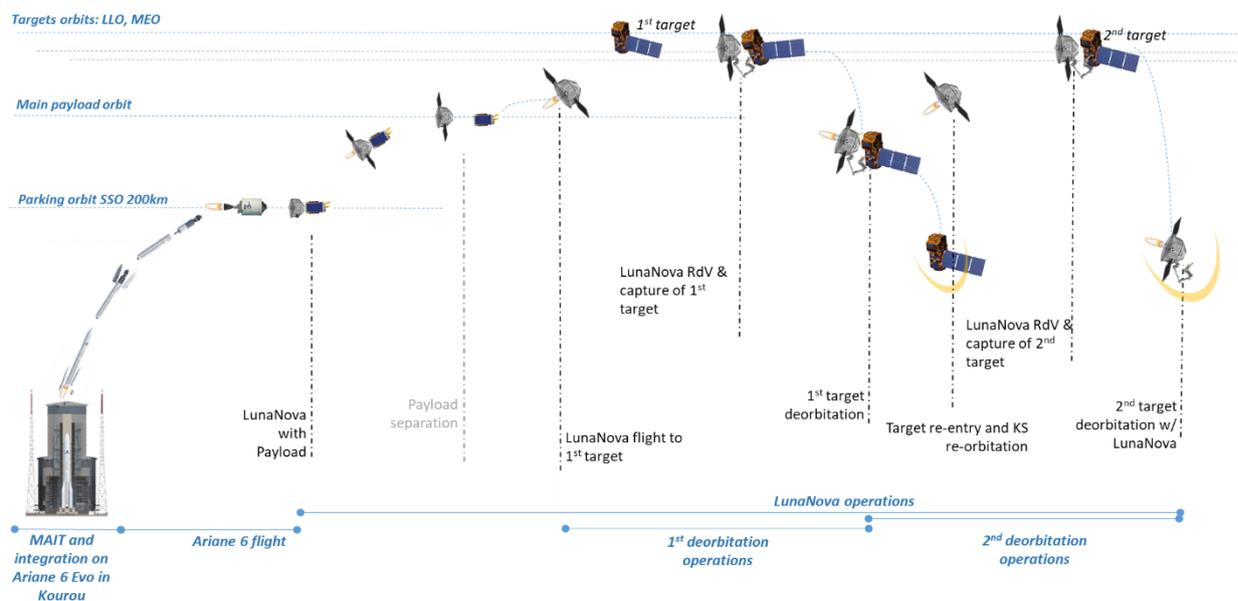
Figure 1: LN Active Debris Removal Service
