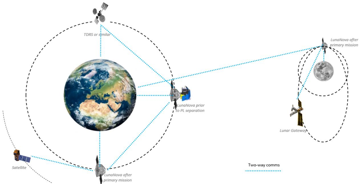
Figure 3: LN Communications Relay Service
