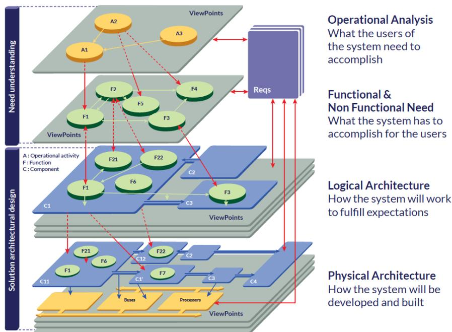
Figure 4: Arcadia working principle
