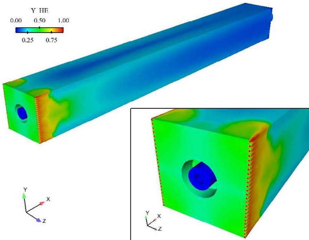
Figure 6 : Helium mass fraction in the chamber
