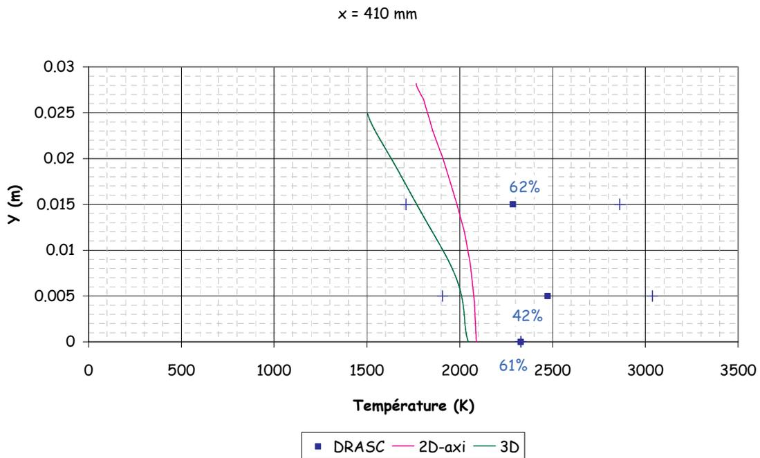
Figure 13 : Comparison CARS / simulation 2D and 3D (X = 410 mm)
