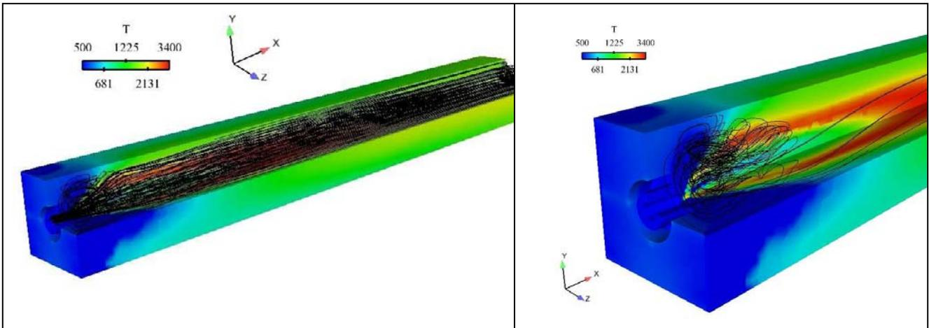
Figure 5 : Stream-line in the chamber
