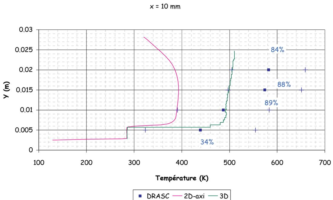
Figure 11 : Comparison CARS / simulation 2D and 3D (X = 10 mm)
