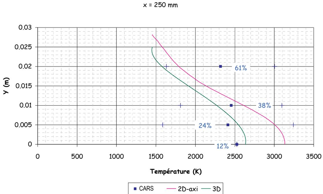
Figure 12 : Comparison CARS / simulation 2D and 3D (X = 250 mm)
