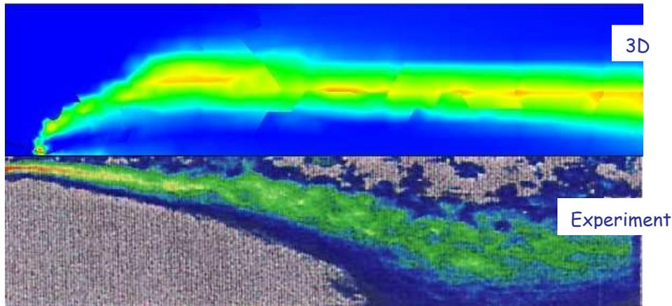
Figure 14 : OH mass fraction (Observation plan)
