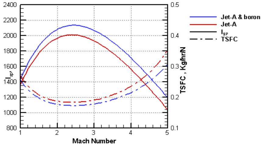
Figure 8. Ideal Ramjet performance for two fuel mixtures with the overall Fuel-to-Air ratio set to 0.04.
