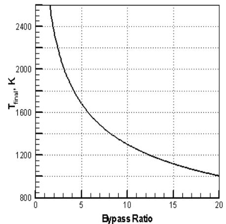
Figure 7 . Temperature reached after adding bypass air to the boron-fuel mixture combustion products as a function of the bypass ratio.
