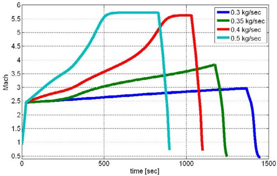
Figure 22. Mach number trajectory for various fuel mass flows, when the fuel mass flow is held constant.
