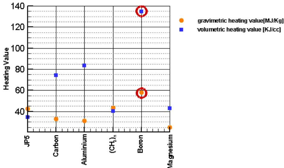
Figure 4. The heat of combustion of various fuels.
