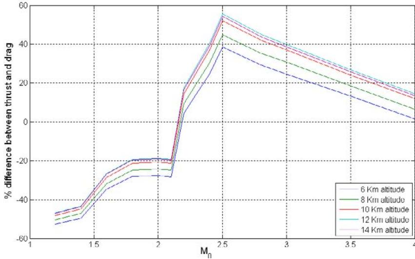
Figure 15. Performance of inlet designed for Mach 2.5.
