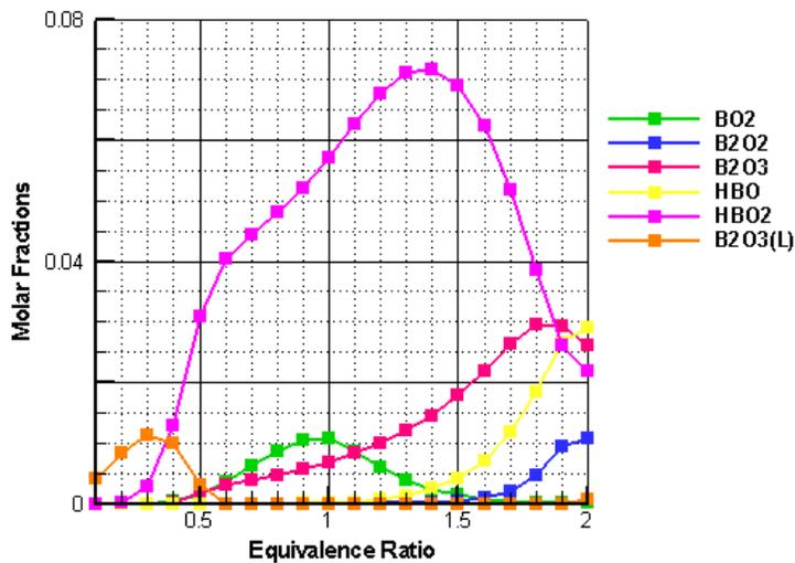
Figure 6. Molar fractions of boron compounds as a function of equivalence ratio.
