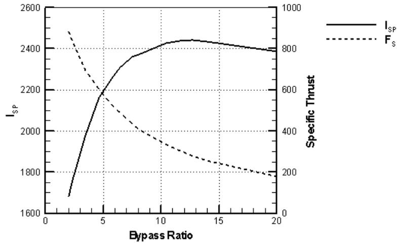
Figure 9. Ideal ramjet performance parameters at 12 km for various bypass ratios.
