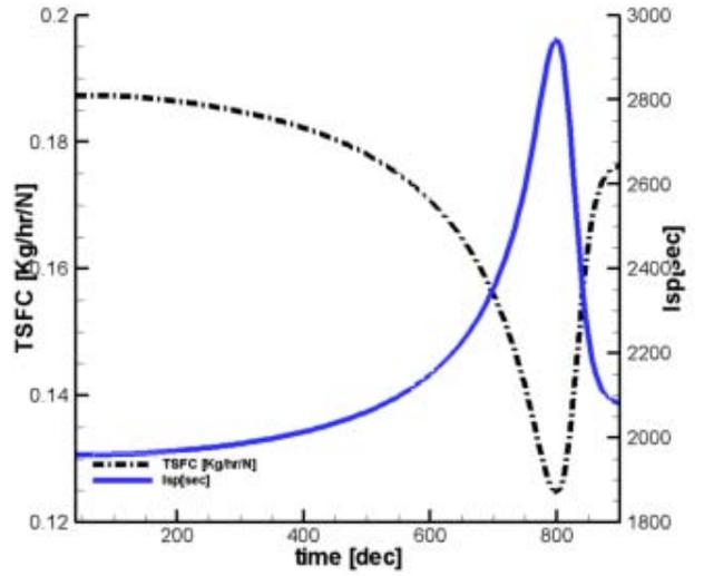
Figure 18. Specific impulse and thrust specific fuel consumption during sustain. for the constant air-to-fuel ratio case.
