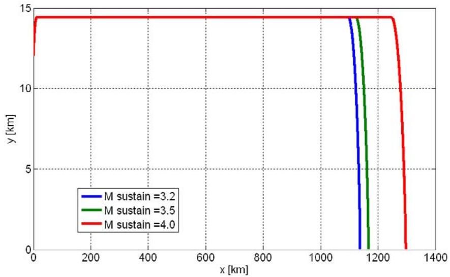
Figure 25. Trajectories for various sustain Mach numbers ,when both the fuel mass flow and the fuel-to-air ratio vary.
