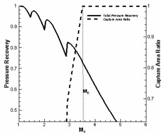
**Figure 14.** Off-design performance of an inlet designed for Mach = 3.5.
