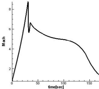
**Figure 3. Mach profile of SRM powered missile.**
