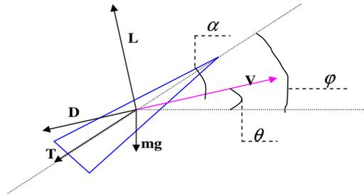
Figure 1. The model used for the trajectory simulation.
