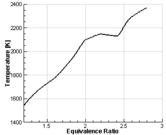
Figure 11. Final temperature variation as a function of various equivalence ratios with a bypass ratio = 2.9.
