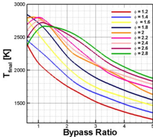
Figure 10. Temperature at the end of combustion vs. the bypass ratio for various first step equivalence ratios.
