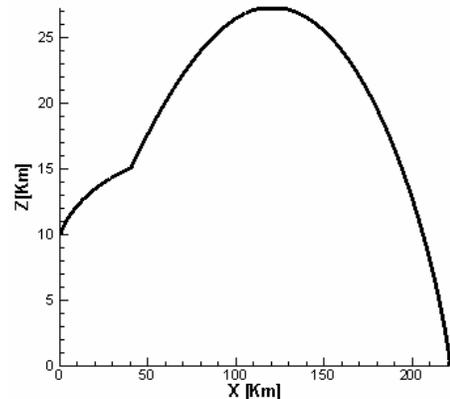
**Figure 2. Trajectory of SRM powered missile.**
