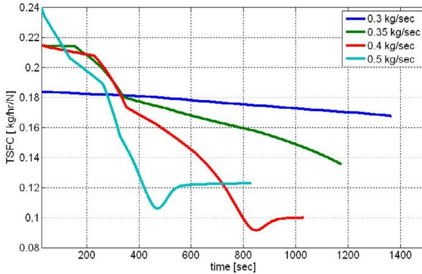
**Figure 23. TSFC variation for various fuel mass flows, when the fuel mass flow is held constant.**
