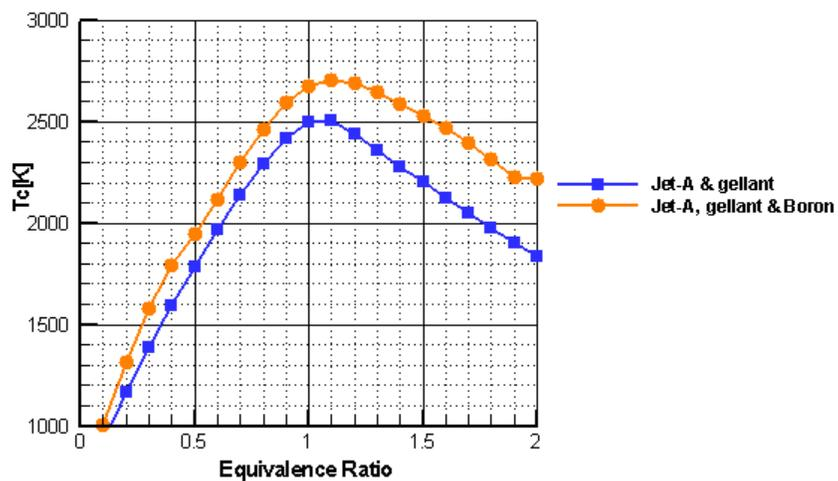
Figure 5 Combustion temperature for two gel fuel mixtures as a function of the equivalence ratio.
