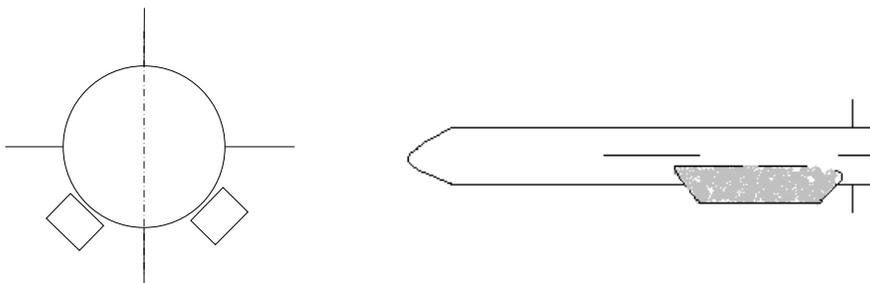
Figure 12. Schematic representation of the missile cross section with two-dimensional twin inlets.
