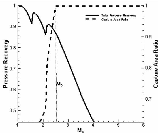
**Figure 13.** Off-design performance of an inlet designed for Mach = 2.5.
