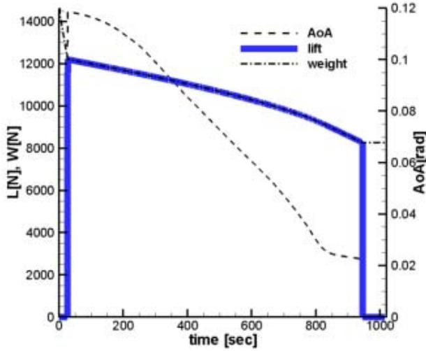
Figure 17 . Angle of attack, lift and weight variation with time for the constant air-to-fuel ratio case.
