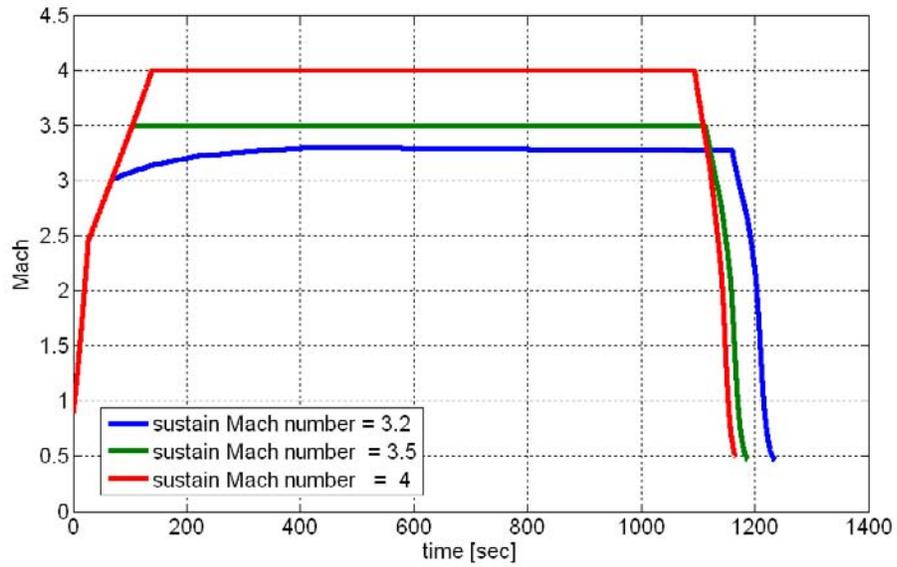
Figure 24. Mach number variation with time , when both the fuel mass flow and the fuel –to-air ratio vary to maintain cruising conditions.
