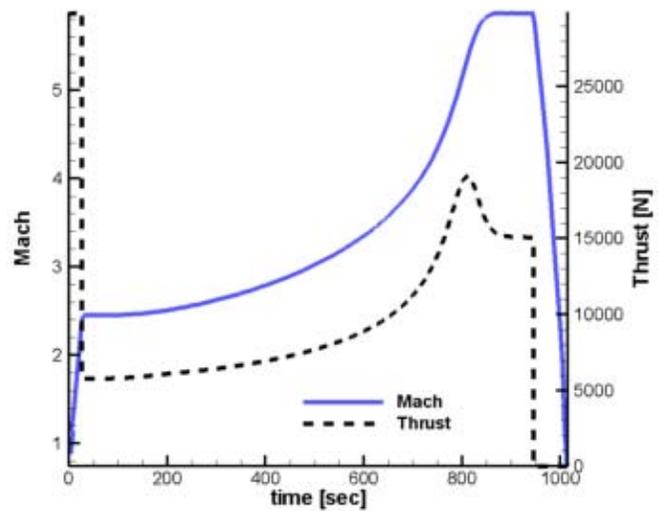
Figure 20. Mach number and thrust profiles for the ramjet powered missile when fuel-to-air is constant.
