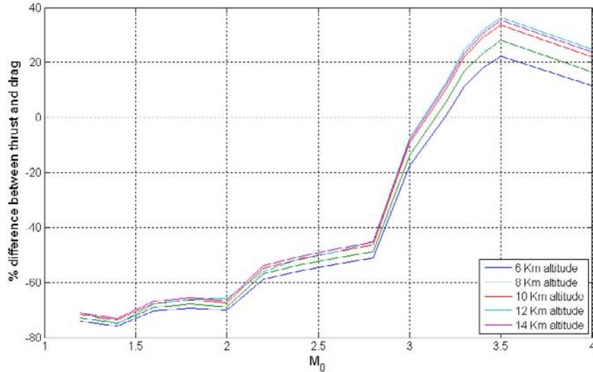
Figure 16. Performance on inlet designed for Mach=3.5.
