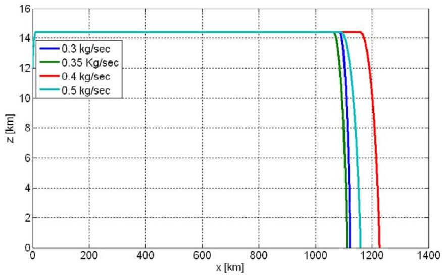
Figure 21. Trajectory for various fuel mass flows, when the fuel mass flow is held constant.
