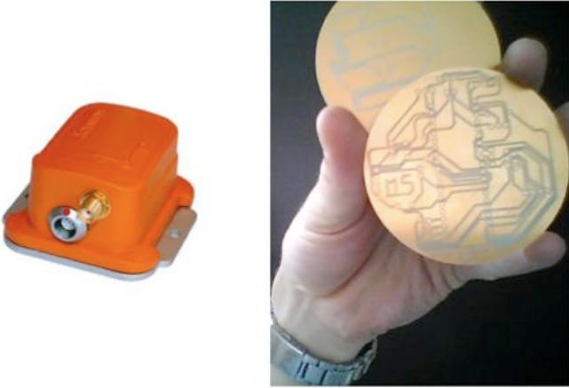
**FIG. 19.** MTi-G IRU (orange box) and circular print plates upon which CPUs will be soldered. The circular shape of the print plates increases the useful area available for the electronic components and facilitates the installation and fixation when placed in the cylindrical fuselage.
