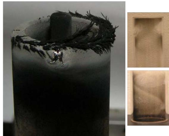
**Figure 14.** Photographs of the deposition on the injector protection (left) and on the walls of the quartz tube (right).
