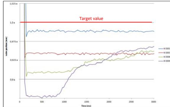
Figure 12: Setting of the  $K_I$ -value (deceleration)
