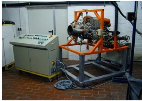
Figure 2: APU GTCP 36-300 in mobile test rig
