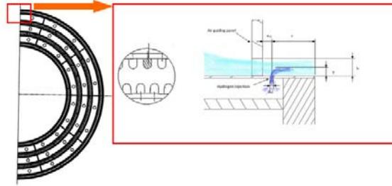
Figure 1: Micromix combustion principle
