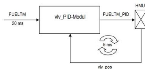
Figure 4: The control loop
