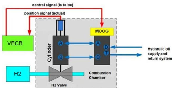
Figure 3: The hydrogen metering unit
