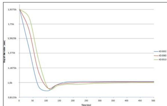
Figure 10: Setting of the  $K_D$ -value (deceleration)
