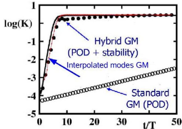
Figure 2: Transients of Galerkin models for flow around a circular cylinder. Improvement - hybrid model and continuous mode interpolation
