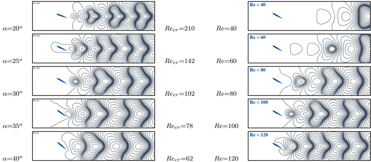
Figure 1: Left: Streamlines of the most unstable modes corresponding to critical Reynolds numbers at different angles of attack. Right: The evolution of the most unstable eigenmodes with the growth of Reynolds number for  $\alpha = 30^\circ$ . On the figure, the streamlines are visualised
