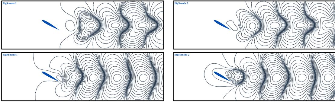
Figure 6: The most dominant eigenmodes based on steady solution (top,  $\lambda = -0.147 \pm 0.720i$ ) and time-averaged solution (bottom,  $\lambda = 0.018 \pm 0.915i$ )
