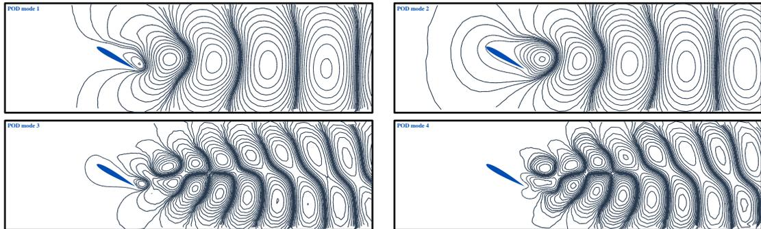
Figure 5: First 4 POD modes used in Galerkin modelling
