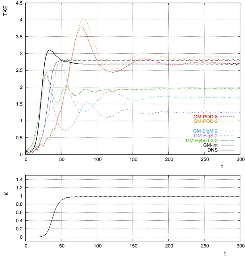
Figure 8: The variation of disturbance kinetic energy (TKE) for different Galerkin models and interpolation parameter  $\kappa$  in function of time, for transition from steady state to the limit cycle oscillation
