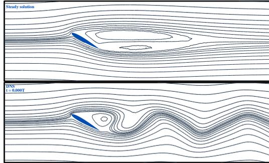
Figure 4: Flow around NACA-0012 airfoil. Top: streamlines of the steady solution. Bottom: streamlines of the snapshot from the periodic (limit-cycle) flow.
