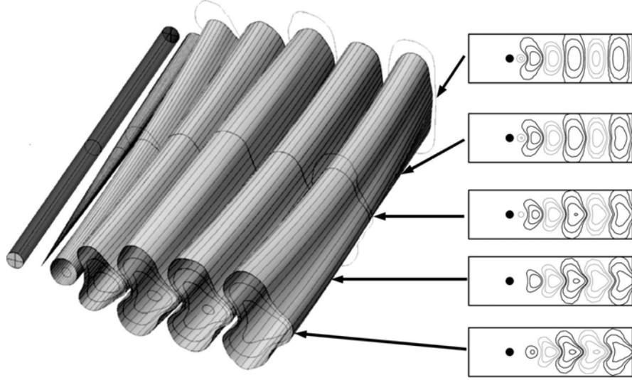
Figure 3: Principal sketch of continuous mode interpolation. Left: Transition between stability eigenmodes and POD modes. Right: streamlines of the intermediate states
