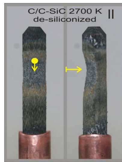
Fig. 11: C/C-SiC sample (II) after tests (2700 K)
