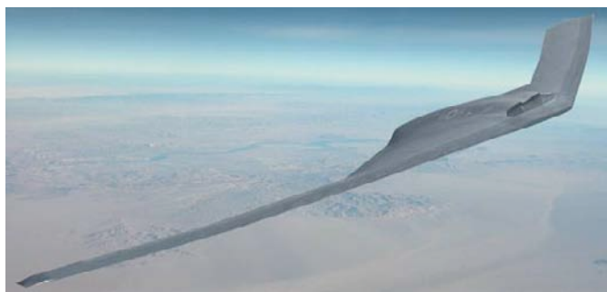
Figure 1 SensorCraft concept designed for laminar flow
