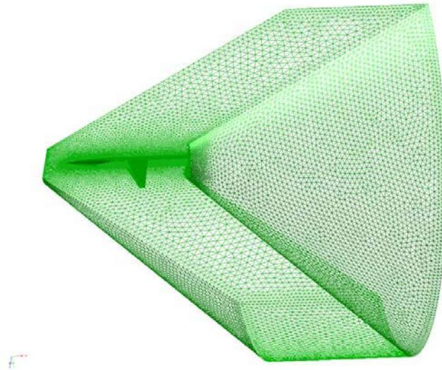
Figure 7: Mesh visualization for analysis at cruise condition
