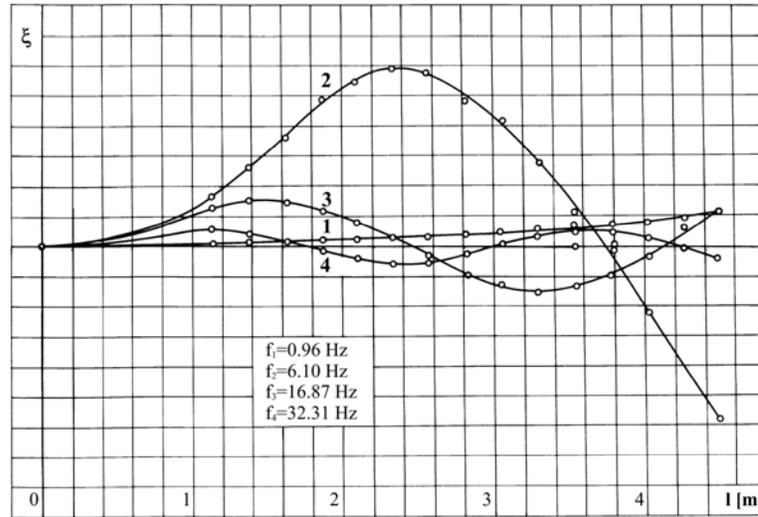
Fig. 5: Natural modes of oscillation for the blade with Rohacell polyurethane foam core (Model 1)
