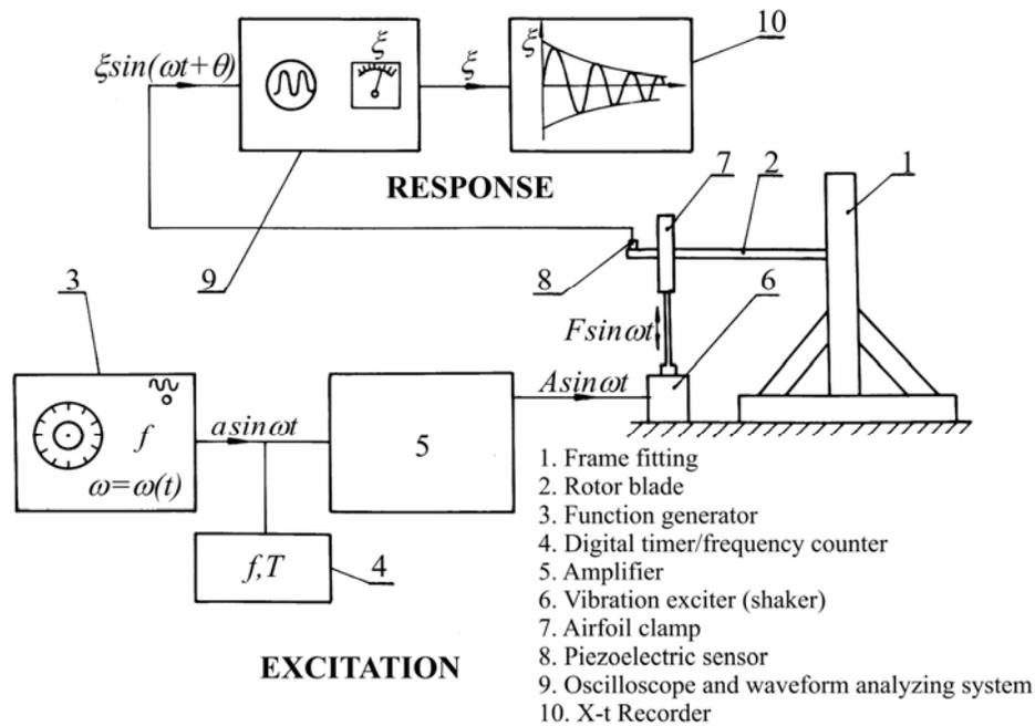
Fig. 4: Employed equipment in vibratory testing
