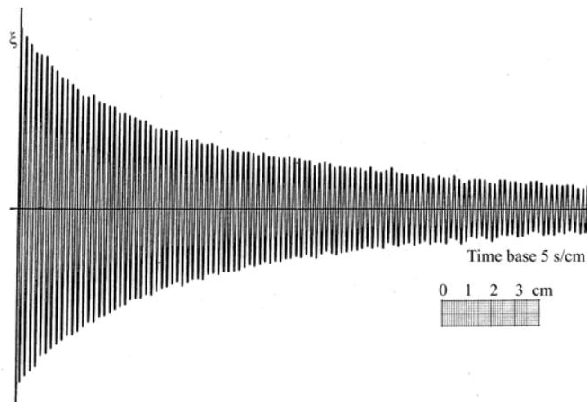
Fig. 10: Structural damping for the blade with Nomex phenolic honeycomb core (Model 3)
