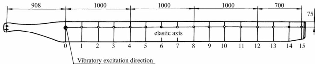
Fig. 3: Measurement points in vibratory testing
