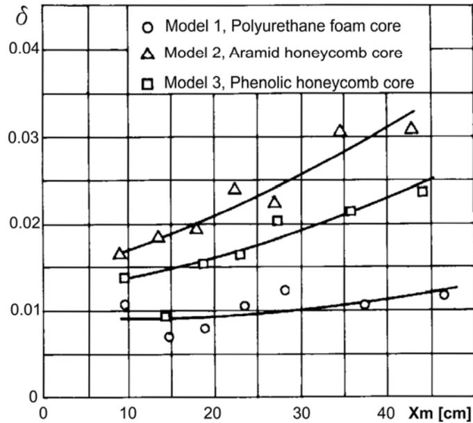
Fig. 11: Logarithmic decrement of blade free vibration
