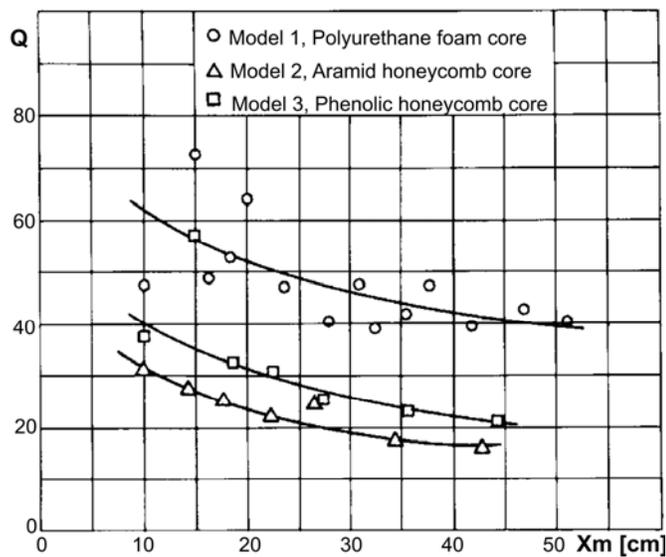
Fig. 12:  $Q$ -factor of blade vibration for all three types of models
