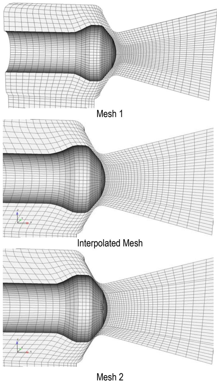
Figure 3 : interpolated mesh between mesh 1 and mesh 2.
