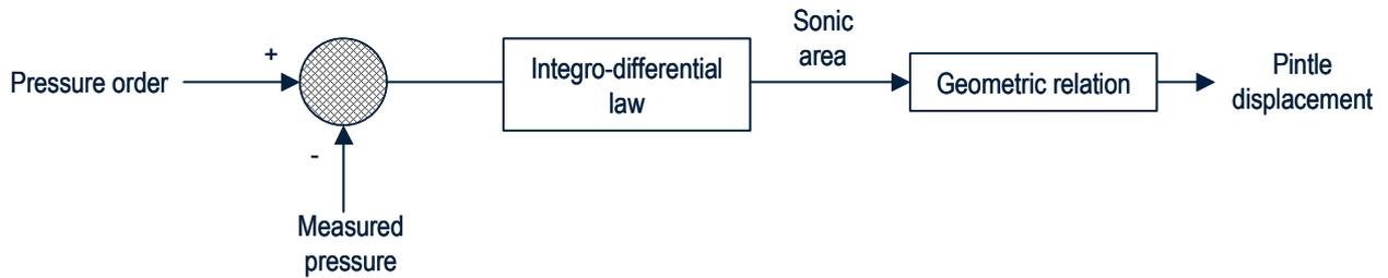
Figure 4 : principle of the control algorithm.
