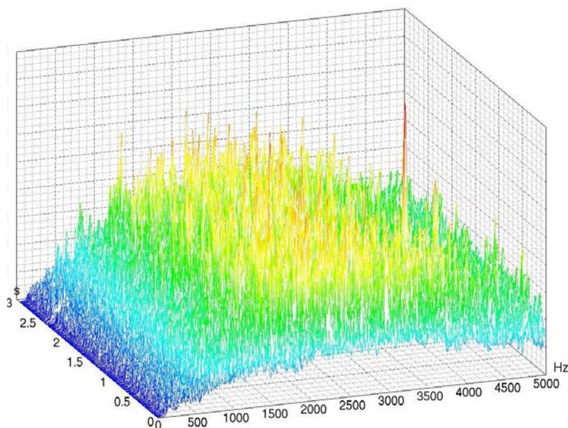
Figure 8 : SRS3D of the experimental pressure signal.
