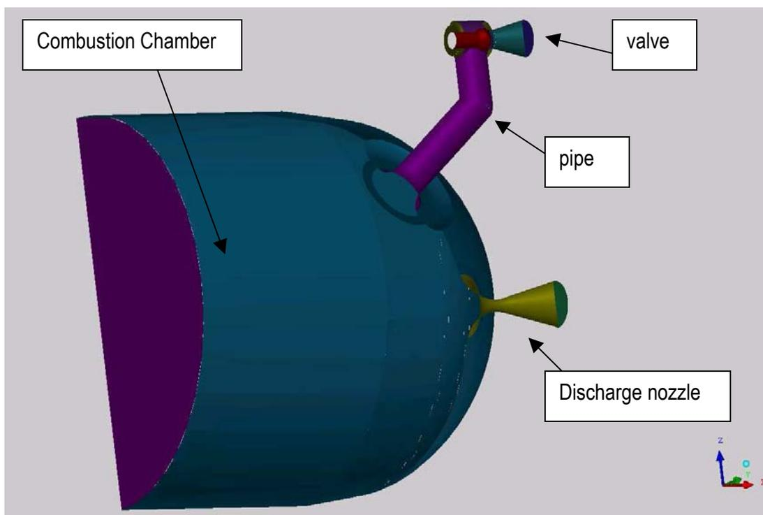
Figure 5 : Design of the experimental device.
