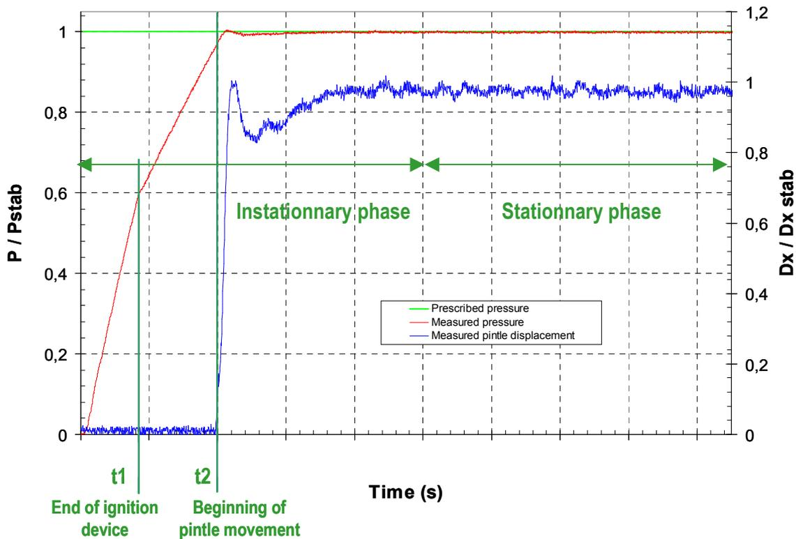
Figure 6 : Experimental results in term of chamber pressure and pintle displacement.
