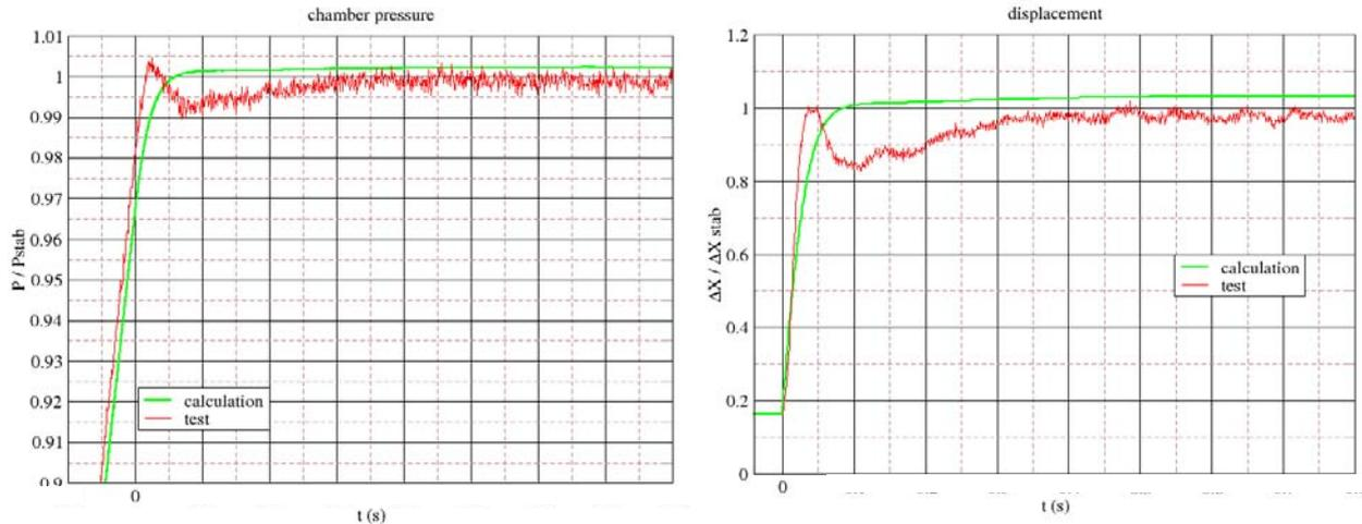
Figure 7 : Time evolution. Left: chamber pressure. Right: pintle displacement.
