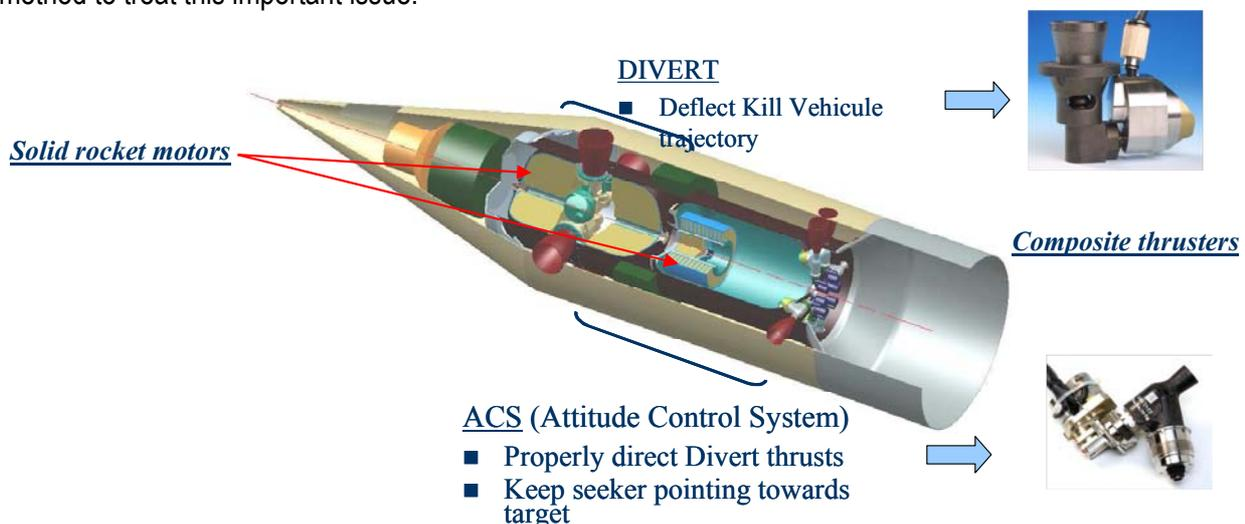
Figure 1 : Solid DACS design for Kill Vehicle.
