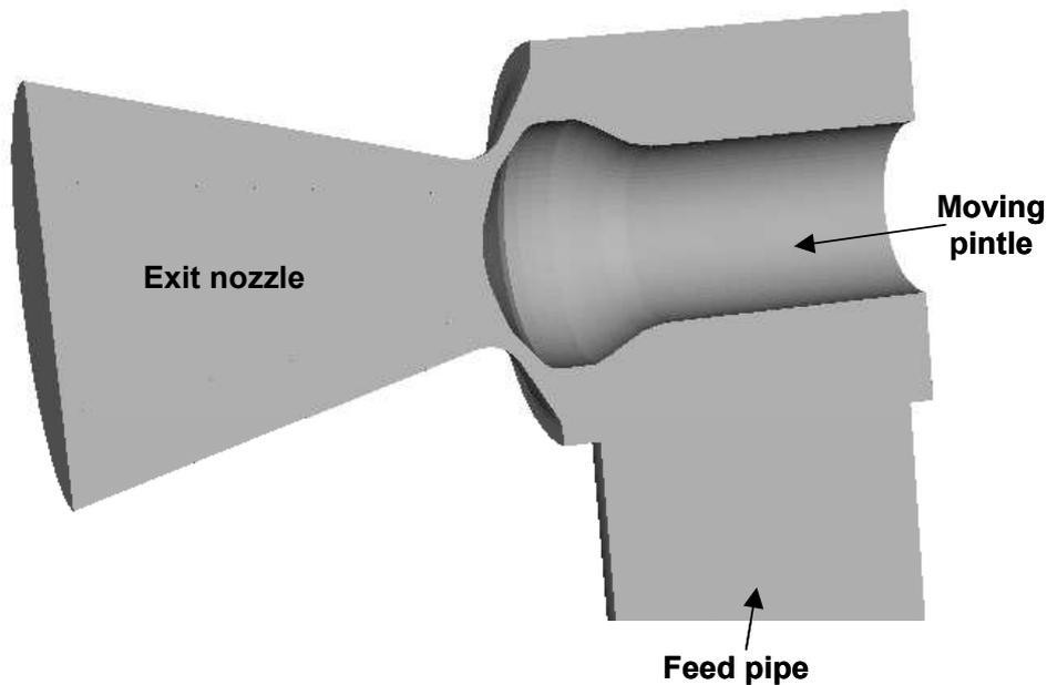
Figure 2 : valve's principle structure.
