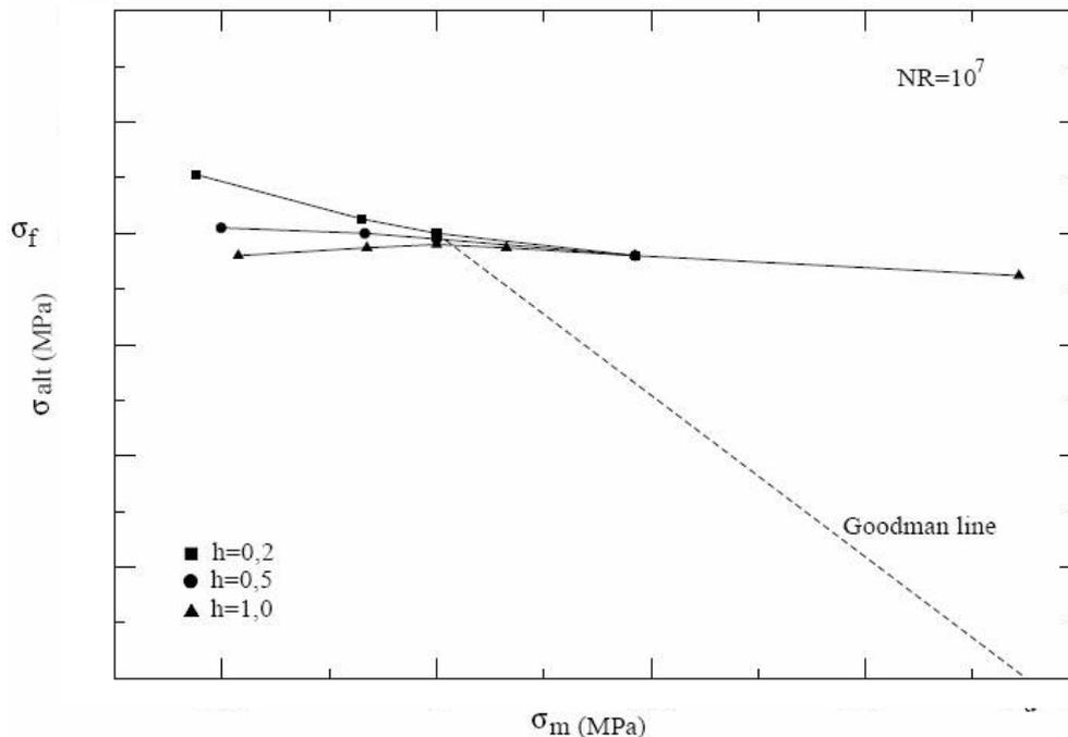
Figure 2 - Influence of the micro-defects closure parameter  $h$  on a Haigh diagram.
