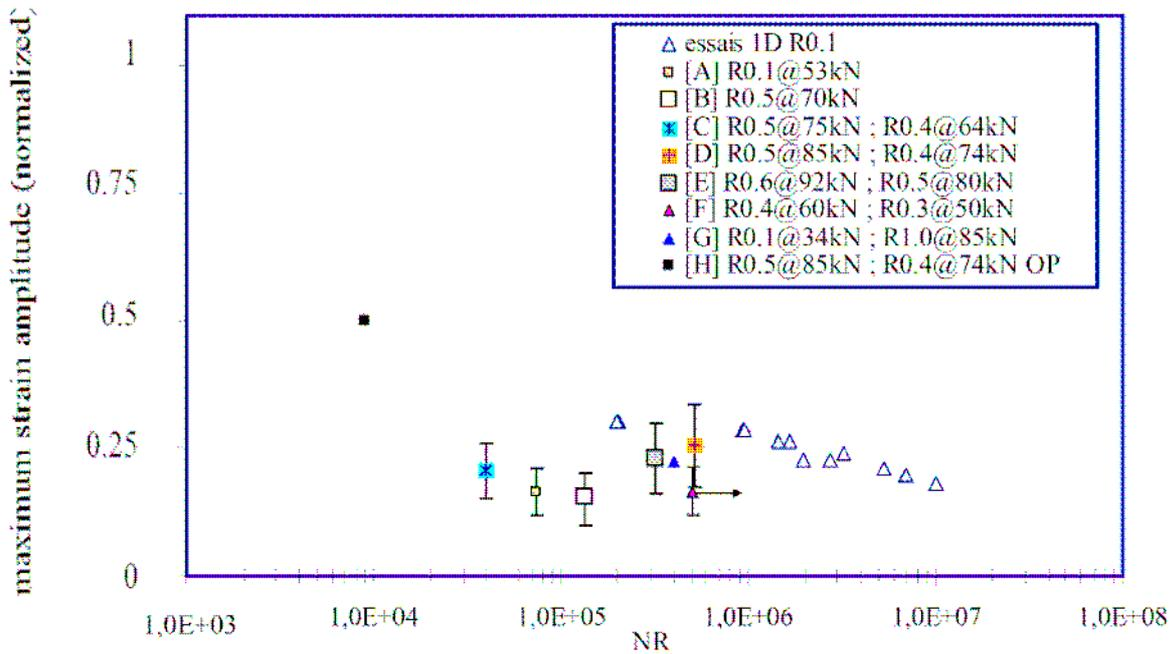
Figure 6. : Summary of biaxial fatigue results for titanium alloy (A, B, C and F tests specimen geometries are thicker).
