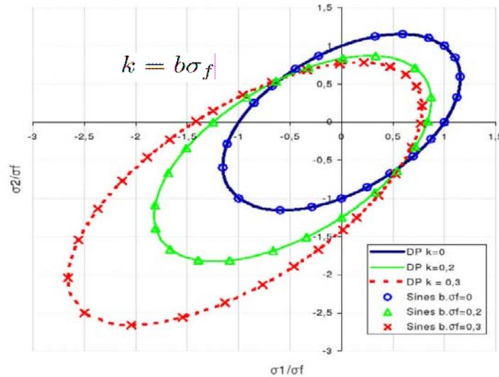
Figure 3 - Ellipsis obtained for Sines criterion and for the 2 scale model modified yield function, for biaxial loadings.
