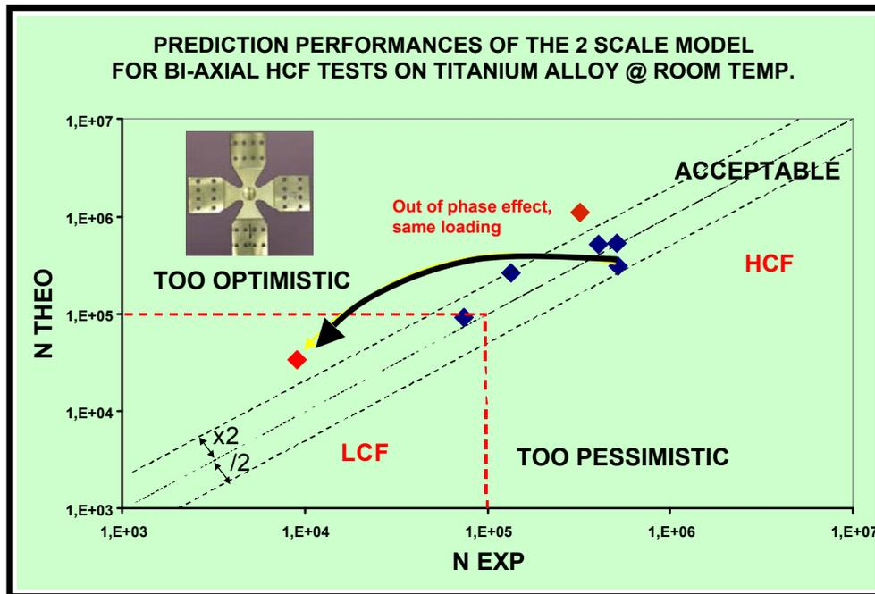
Figure 7. : Comparison between predicted and experimental values for titanium alloy.
