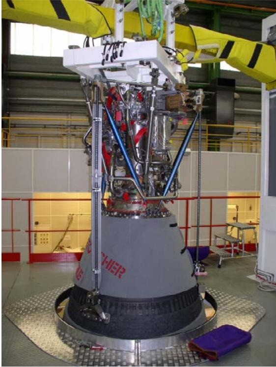
Figure 7 : Engine dynamic testing
