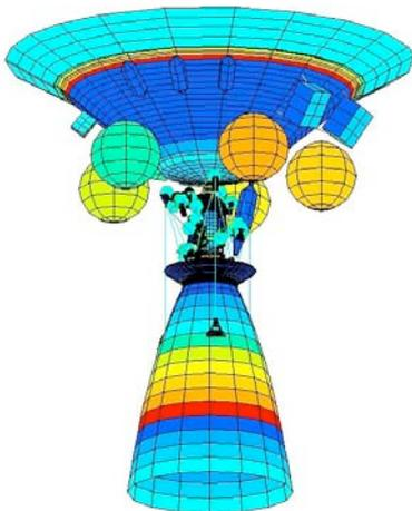
Figure 8 : Thermal model of the engine
