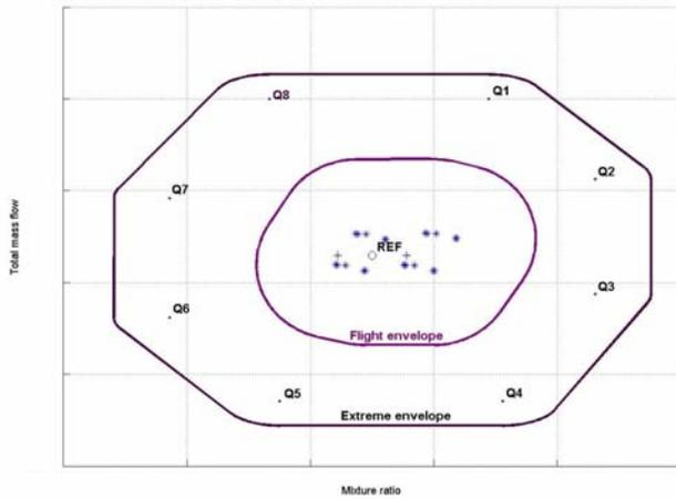
Figure 5 : Engine operating envelopes in the Thrust (or total flow) vs mixture ration axis
