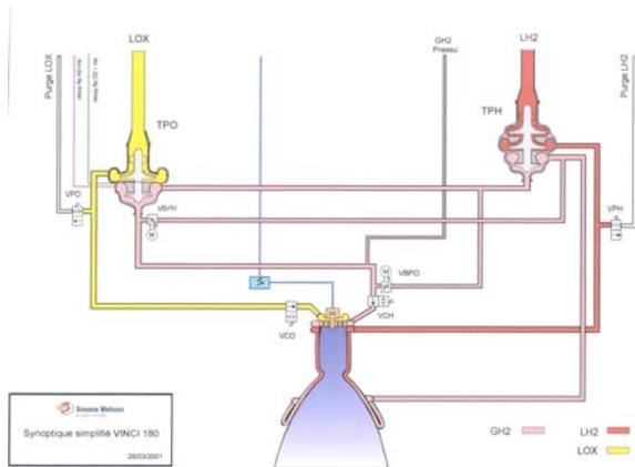
Figure 3 : VINCI flow schematic
