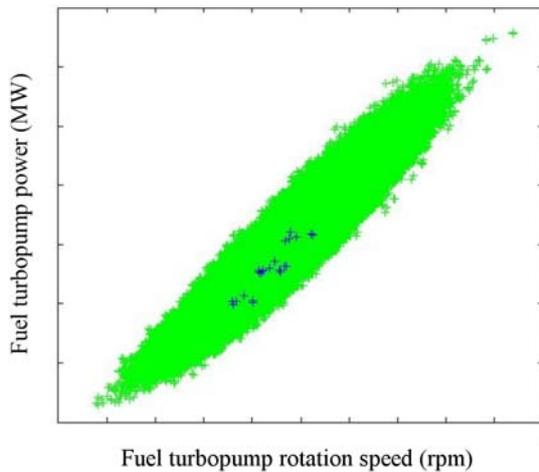
Figure 6 : Fuel turbopump operating domain obtained by Monte-Carlo analysis
