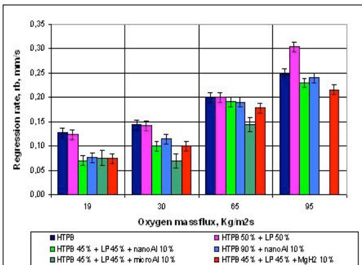
Figure 4. Regression rate results for the selected fuel formulations. Tests performed at 19, 30, 65 and 95  $\text{kg}/\text{m}^2\text{s}$  oxygen mass flux.  $\mu\text{Al}$  formulation tested only up to 65  $\text{kg}/\text{m}^2\text{s}$ .
