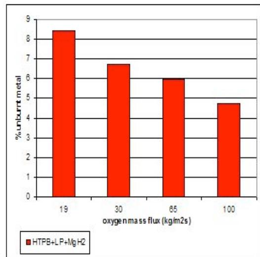
Figure 5. Percentage of unburnt metal over the metal content, as a function of oxygen mass flux, for the magnesium hydride filled formulation.
