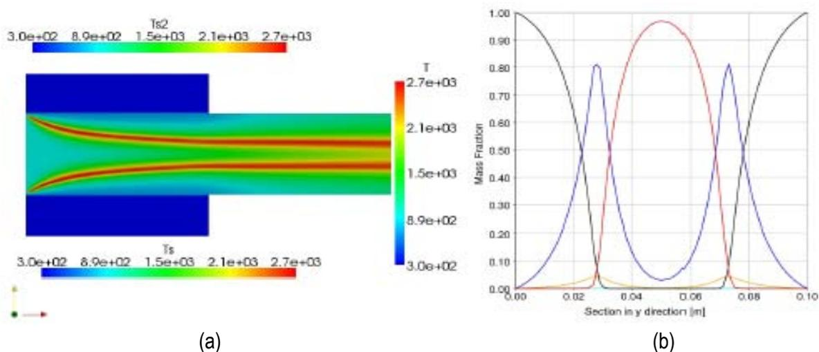
Figure 8. Numerical simulation results for a 2D slab combustion chamber. A  $k-\epsilon$  turbulence model, a four reactions kinetic scheme and a radiation model are taken into account. (a): temperature field; the blue regions represent the two solid fuel grains; (b) species concentration profiles at a cross section of the chamber located at 45% of the grain length.
