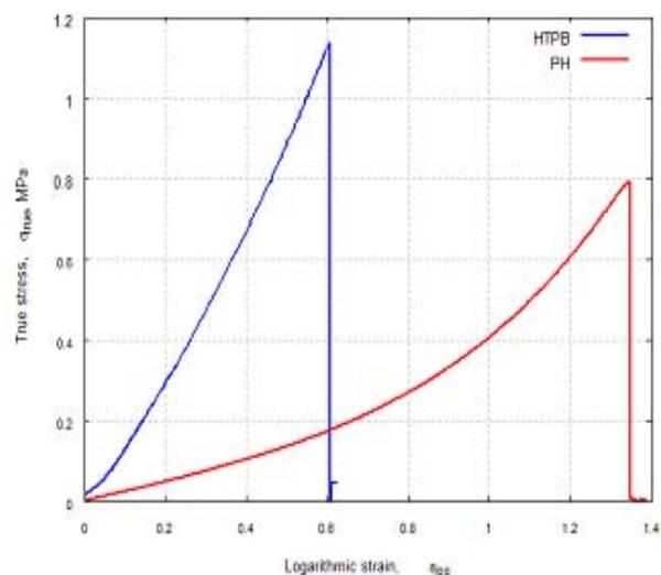
Figure 7. True stress vs. logarithmic strain for HTPB- four based and HTPB-paraffin mixed formulations.
