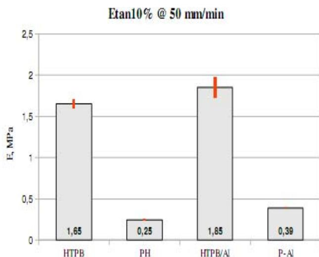
Figure 6. Tangent elastic modulus at 10% (ASTM 111) for different formulations, metallized or not.
