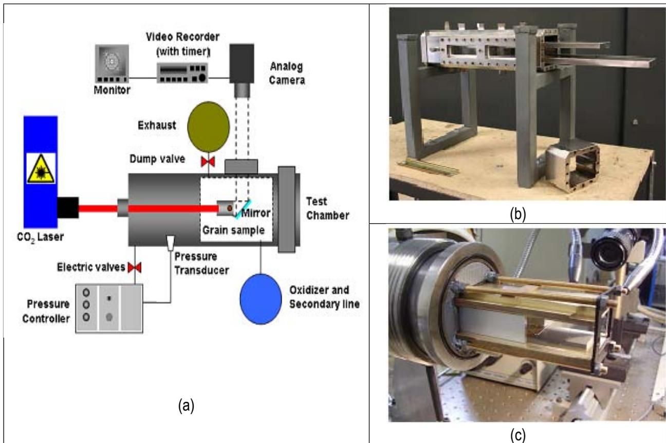
Figure 2. SPLab testing facilities.
