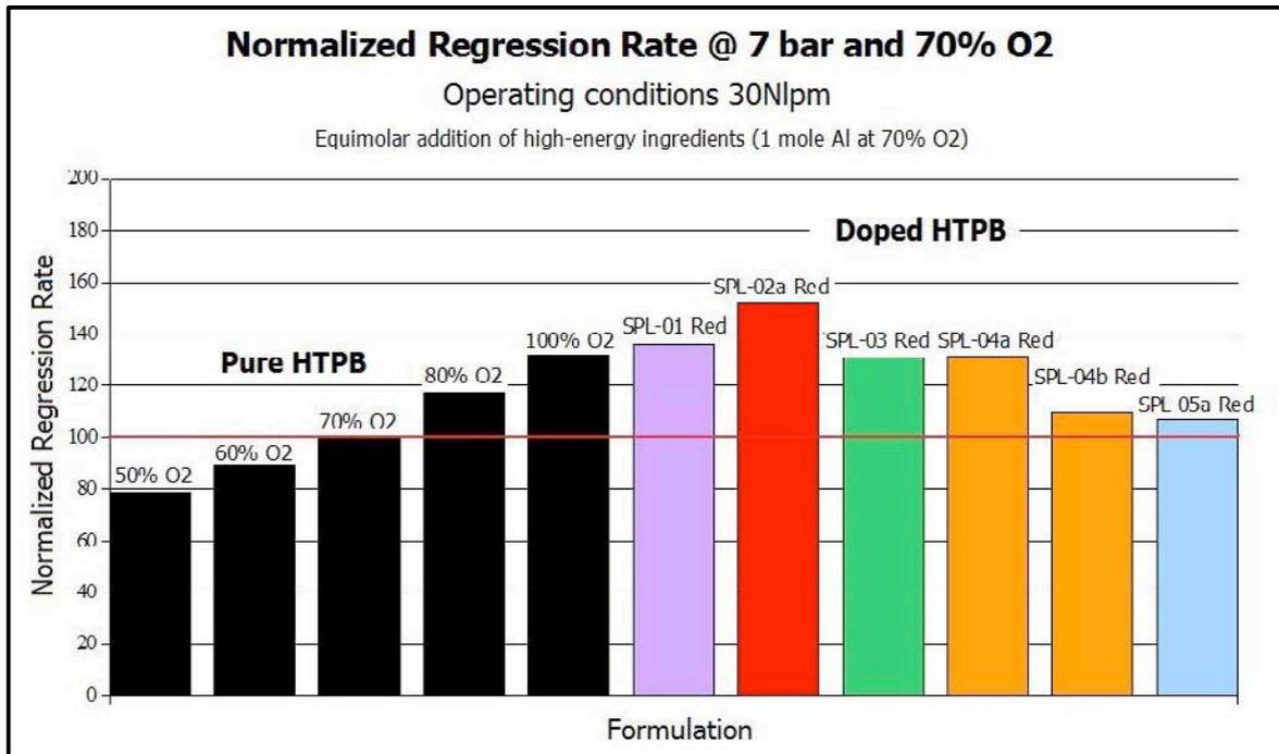
Figure 3a. Normalized regression rates for a variety of HTPB-based solid fuels at 7 bar and 70% O<sub>2</sub>.
