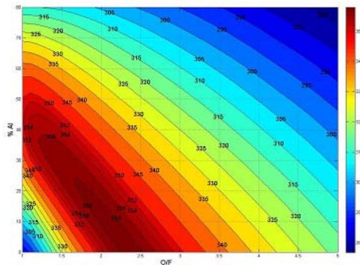
Figure 1. Specific Impulse [s] for HTPB, Al, O<sub>2</sub>: shifting equilibrium model.
