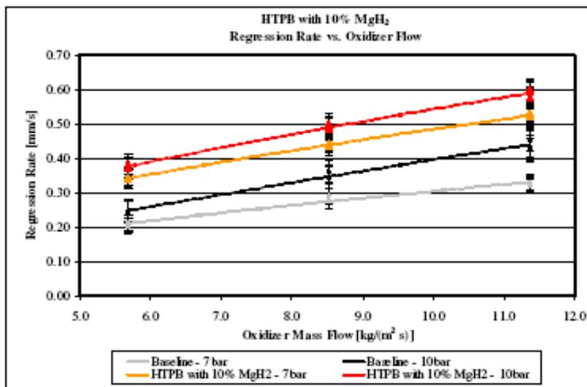
Figure 3b. Regression rate vs. oxidizer mass flow rate for HTPB loaded with 10% MgH<sub>2</sub>, burning under reference conditions at 7 and 10 bar. Oxygen fraction: 50%. Each operating point defined by 3 tests.
