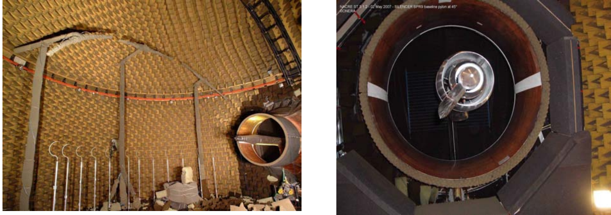
Figure 2: Mock-up of the engine installed in the CEPRA-19 Wind Tunnel.
