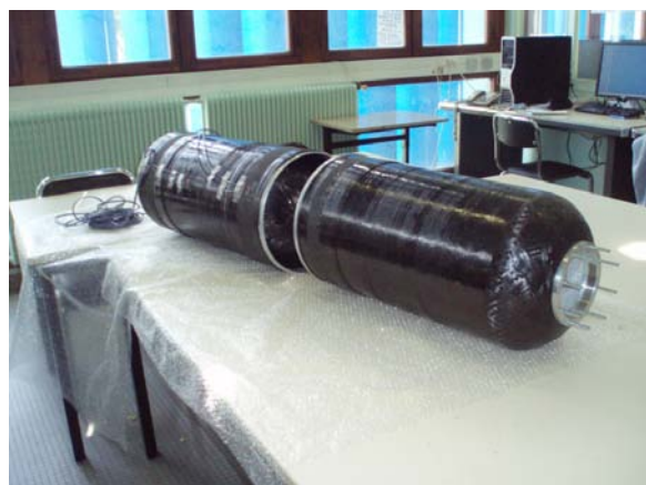
Figure 3: ENSAM 2009 (a) Filament winding of a combustion chamber, (b) Cryogenic tank and combustion chamber
