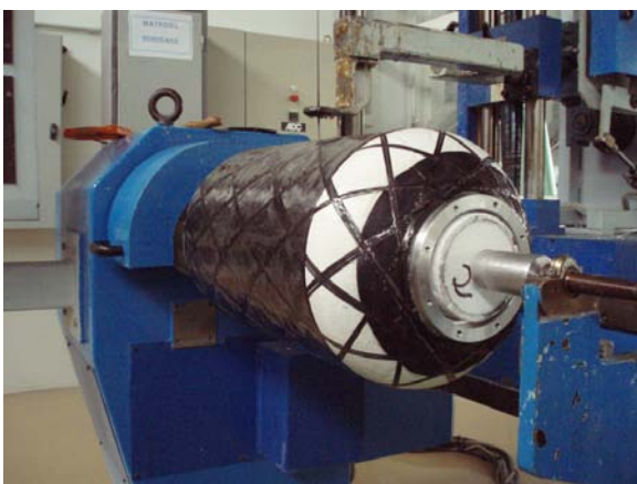
Figure 3: ENSAM 2009 (a) Filament winding of a combustion chamber, (b) Cryogenic tank and combustion chamber
