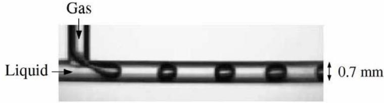
**Figure 3:** Schematics of the bubble generation method.
