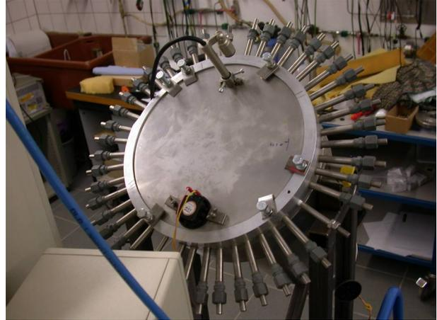
Figure 2: Absorber ring mounted to the steam generator.
