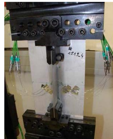
Fig. 2: Specimen in mechanical tensioning set-up equipped with thermocouples.
