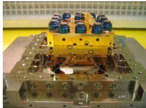
**Figure 7: Accelerometer Sensor Head (ASH-02) ULE core containing the Pt-Rh proof mass. The lower metallic structure is the “sole plate” providing the reference frame interface with the carbon-carbon gradiometer arm.**
