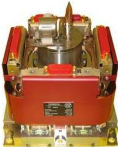
**Figure 8: ASH-05 before delivery to Thales Alenia Space Gradiometer Team. On the top of the ASH, there is the ionic pump used during functional test on ground and the getter housing.**
