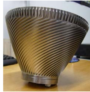
Figure 10: Helical cooling channels of the first part of the nozzle
