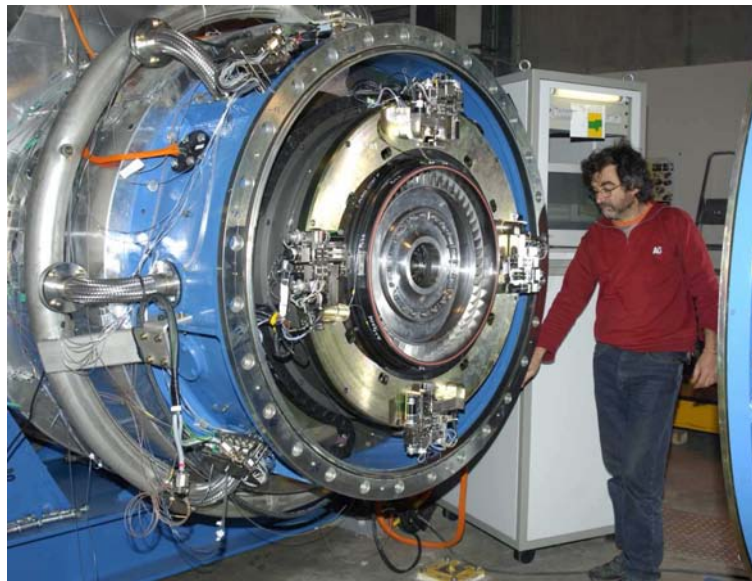
Figure 8. Wake survey system. The system is shown with its 4 modules, as rigged for flow analysis downstream the rotor.
