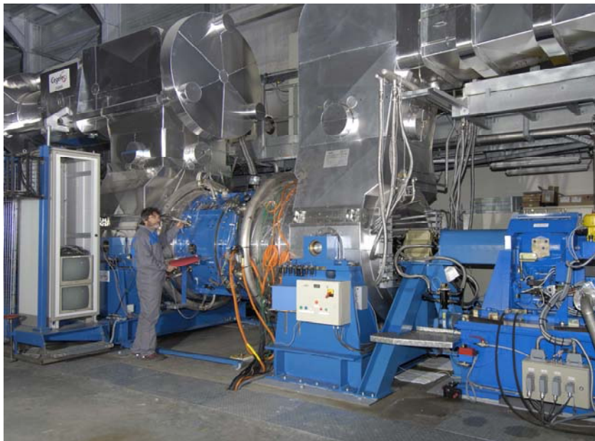
Figure 1. Central part of TURMA. This figure shows the bench in "closed" position, with (from right to left), the duct for HP air supply, the HP shaft line with its torque meter and hydraulic brake, the envelope enclosing the turbine(s) and the measurement systems, and the exhaust duct (LPT exit).
