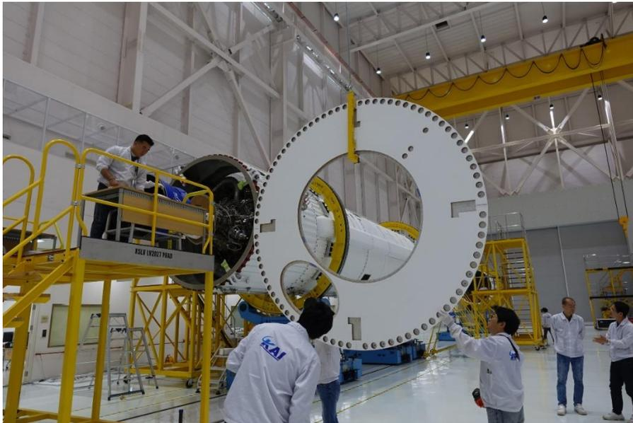
Figure 7 Base plate with the rigid TPS of the TLV
