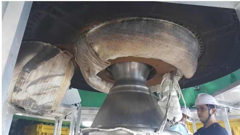
Figure 13 Rigid and flexible TPS after combustion tests
