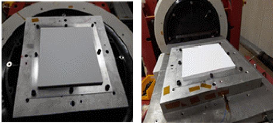
Figure 8 Test specimen mounted on the shaker (Left: vertical direction, Right: horizontal direction)
