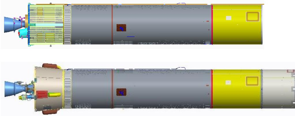
Figure 3 1st stage of the TLV (Up), and 2nd stage of the KSLV-II (Down)
