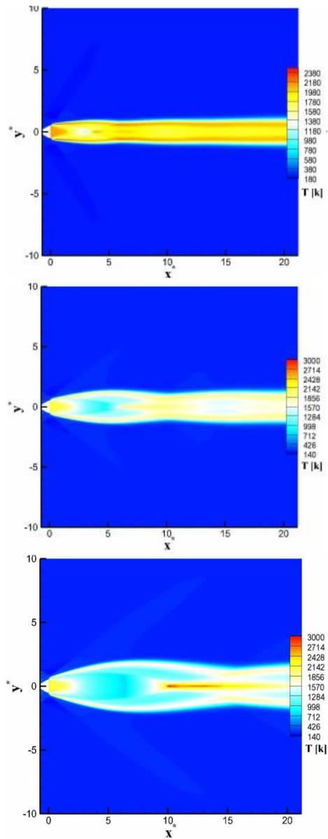
Figure 4 Calculated temperature of plume by CFD analyses (Up: 10km, middle: 15km, Down: 20km)
