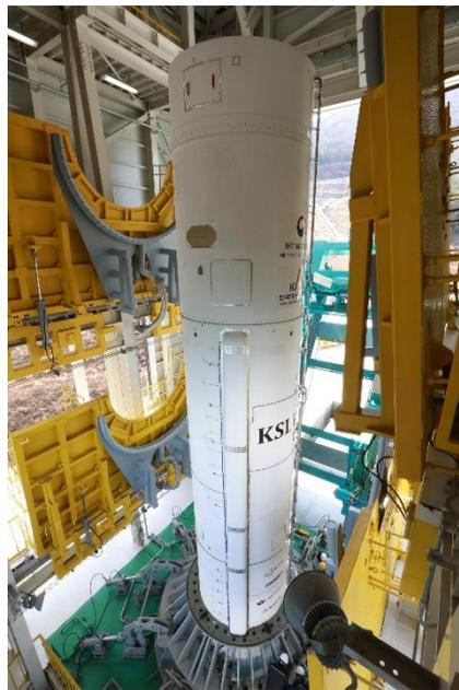
Figure 11 Qualification model of TLV in the test stand for a combustion test
