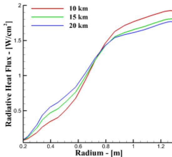
Figure 5 Calculated heat fluxes at the base by CFD analyses[6]
