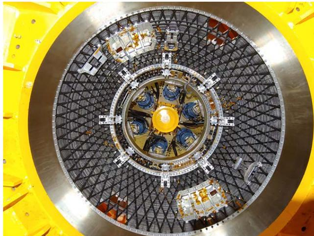
Figure 10: Load introduction during static load test –Bottom view of interstage 2-3
