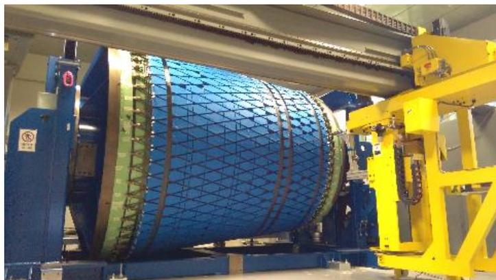
Figure 4: IS 2/3 composite structure during ribs and helixes winding
