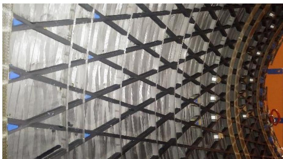
Figure 6: IS 2/3 composite structure after cure (inside view)
