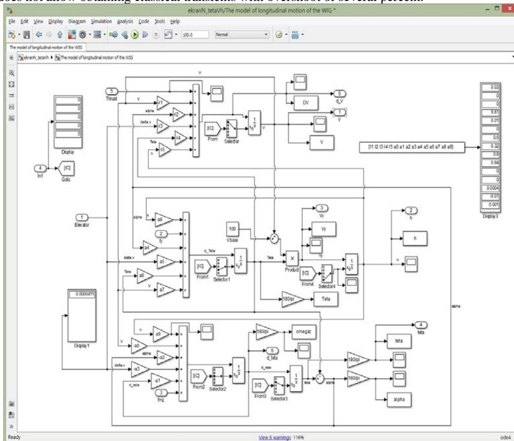
Figure 5: Program for modeling the longitudinal movement of a ground-effect vehicle when flying in the area of the ground effect
