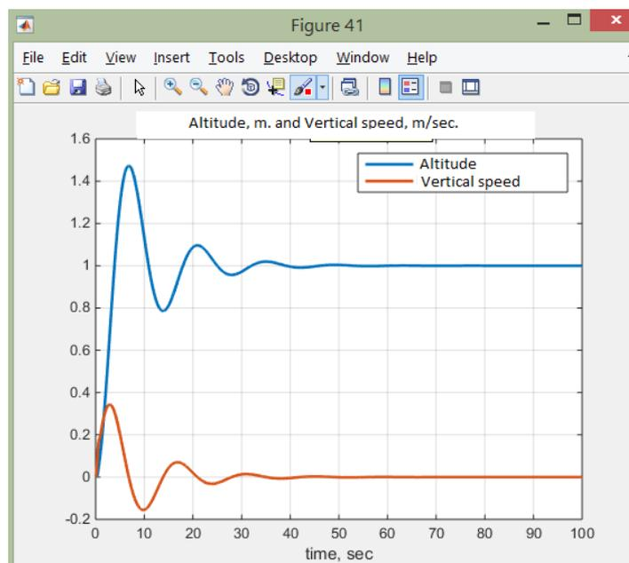
Figure 6: Processes of changing the altitude (blue) and vertical speed (orange) when “jumping” at 1 m
