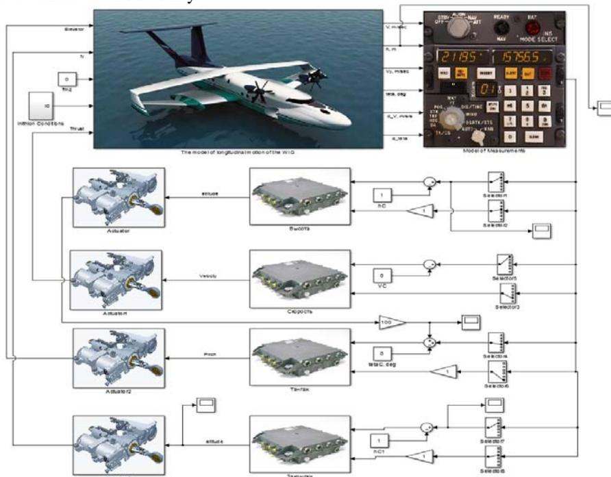
Figure 4: Block diagram of the stabilization system of the ekranoplane angular motion, its altitude and speed when flying in the area of the ground effect
