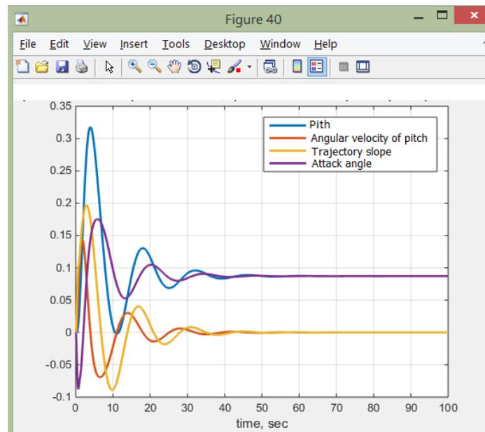
Figure 7: Processes of change in the angular parameters of motion with a “jump” at 1m: pitch (blue), angular velocity of pitch (orange), trajectory slope (yellow), attack angle (purple)
