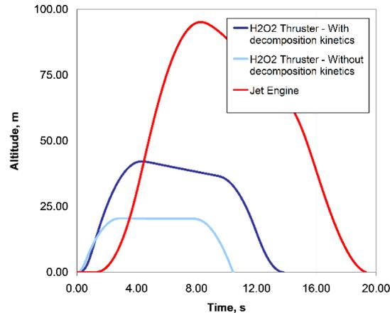
Figure 19 : Computed altitude profiles - Comparisons between jet engine and HTP thruster with infinite or finite decomposition rate
