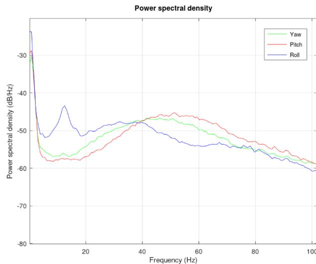
Figure 11 : Gyrometers power spectral density
