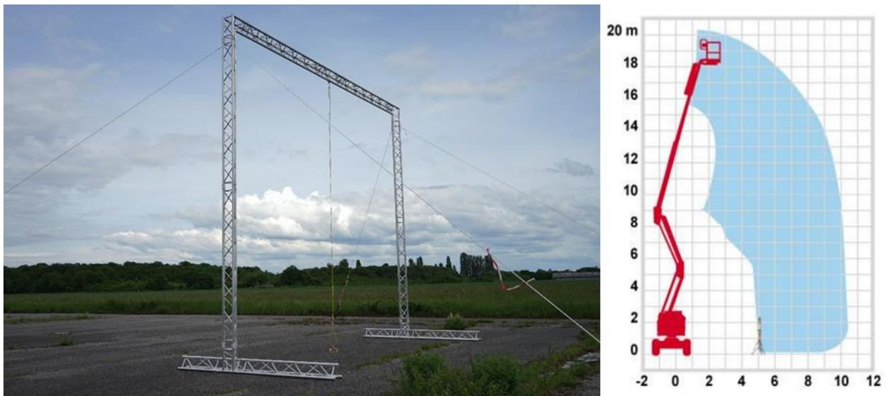
Figure 6 : 6 m fix gantry and 20 m crane for tethered flights
