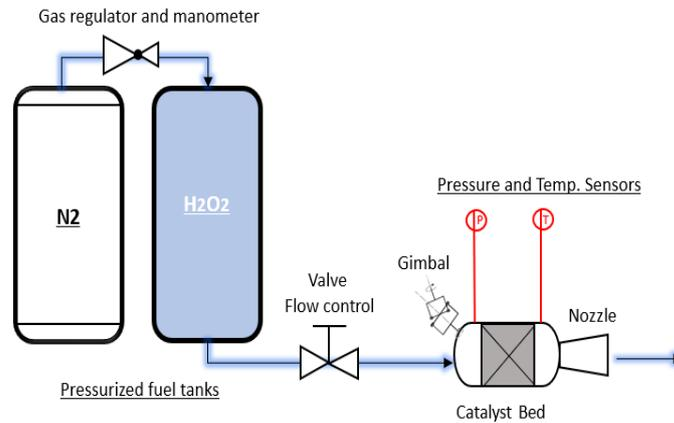
Figure 16 : Conceptual view of the FROG-H motor
