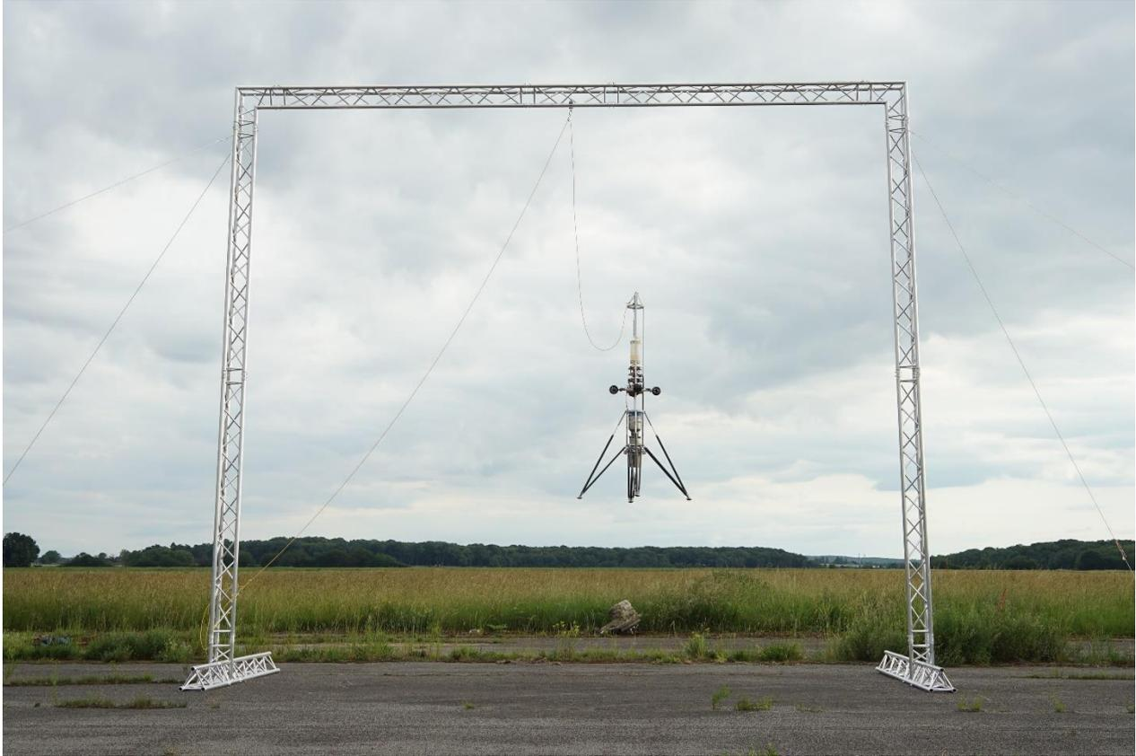
*Figure 15: FROG-T during a tethered flight*
