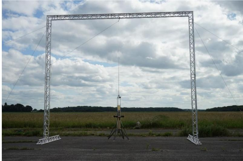
Figure 7: FROG-T tethered to the 6 m fix gantry just before engine ignition
