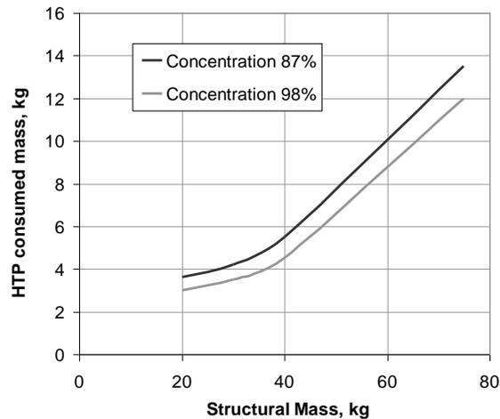
Figure 18: Computed HTP consumption for 87.5% and 98% thrusters and for different flying mass assumptions
