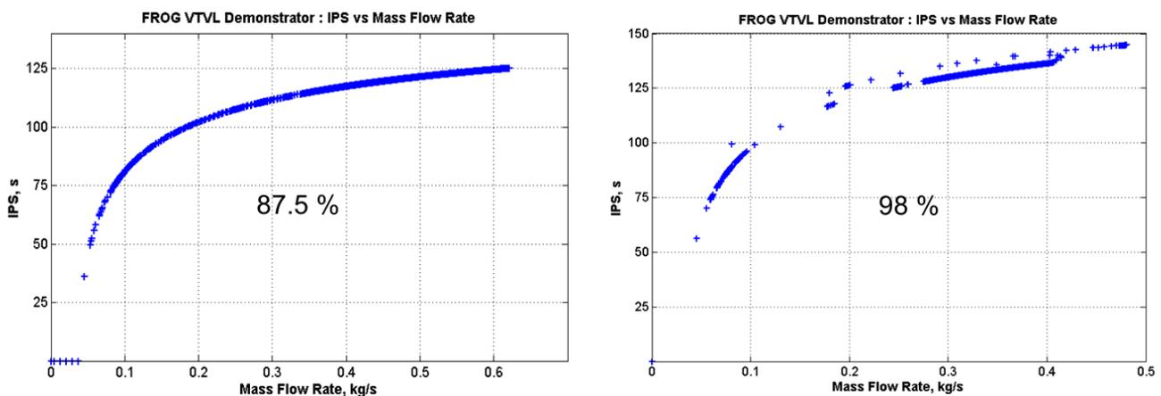
Figure 17: Computed efficiency of 87.5% and 98% HTP thrusters at different flight operation point
