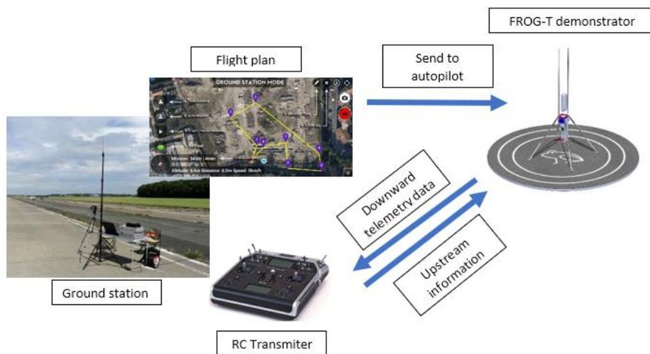
Figure 2 : Ground station and data links
