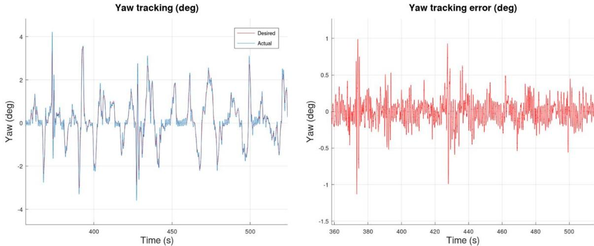
Figure 9 : Yaw tracking (both actual and desired curves are superimposed) and yaw tracking error
