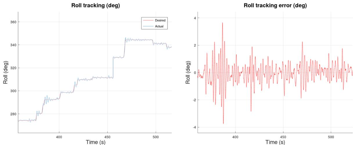
Figure 10 : Roll tracking (both actual and desired curves are superimposed) and roll tracking error
