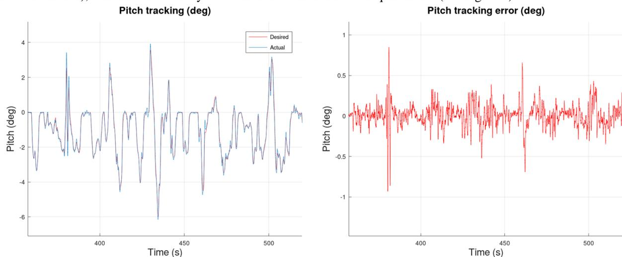
Figure 8: Pitch tracking (both actual and desired curves are superimposed) and pitch tracking error
