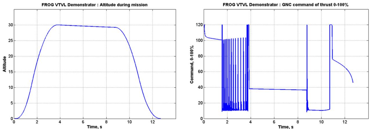
Figure 20 : Computed GNC command of thrust during typical VTVL mission with hovering
