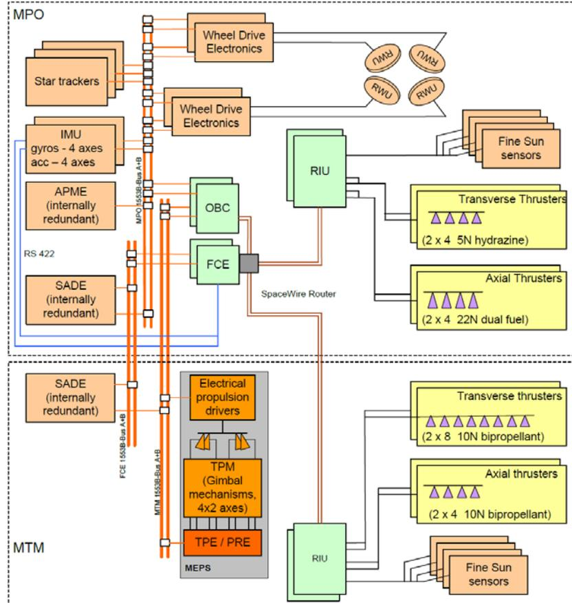
Figure 5: AOCS hardware architecture.
