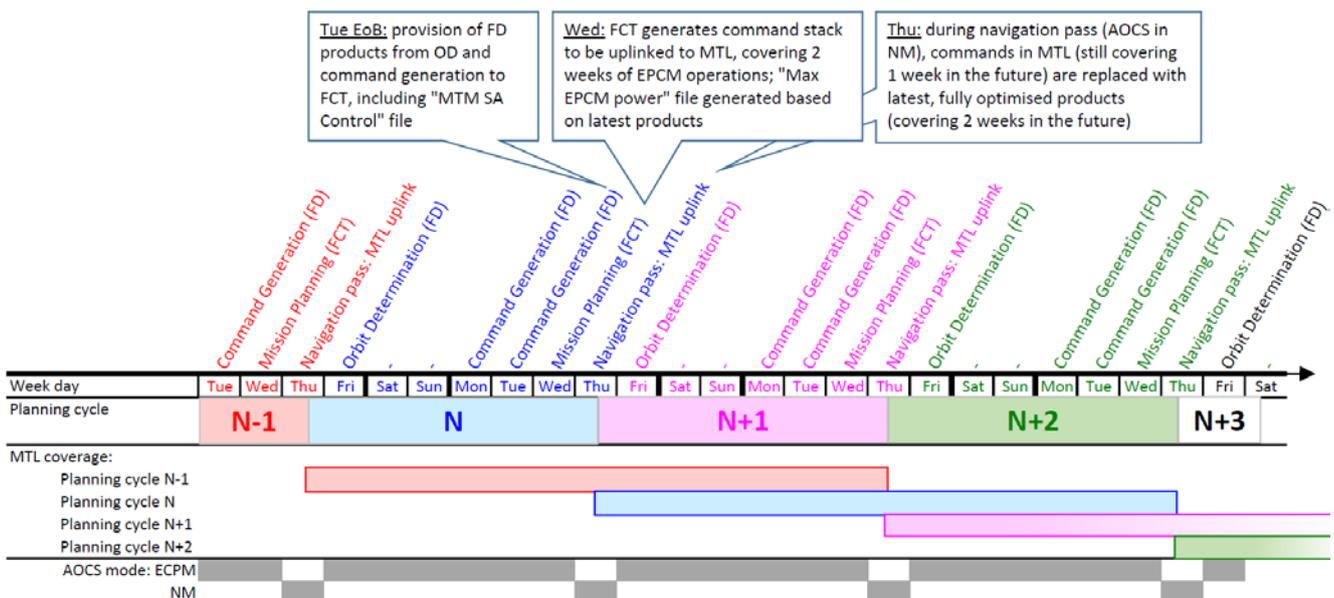
Figure 15: Weekly planning cycle during Electric Propulsion thrust arcs, including special processing for determining the MTM solar array pointing and the corresponding power available for EP thrusting.
