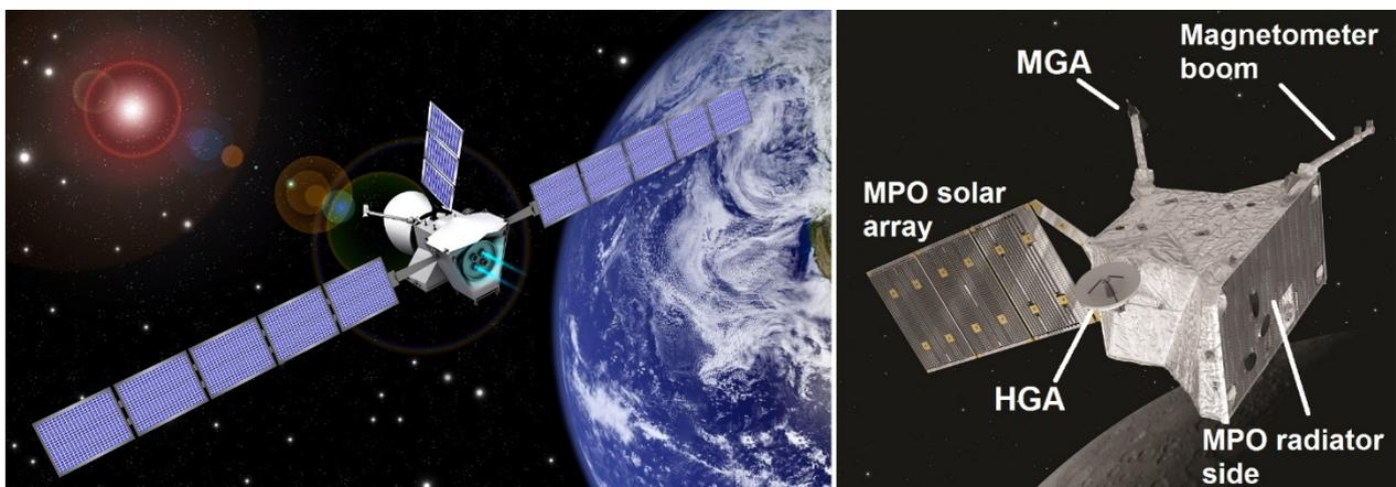
Figure 3: BepiColombo in cruise configuration (left), MPO at Mercury (right).
