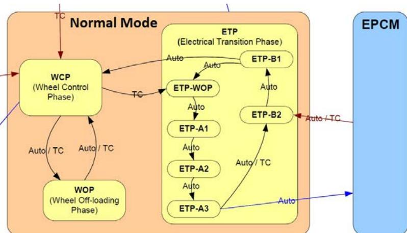
Figure 11: AOCS mode transitions for EPCM entry/exit.
