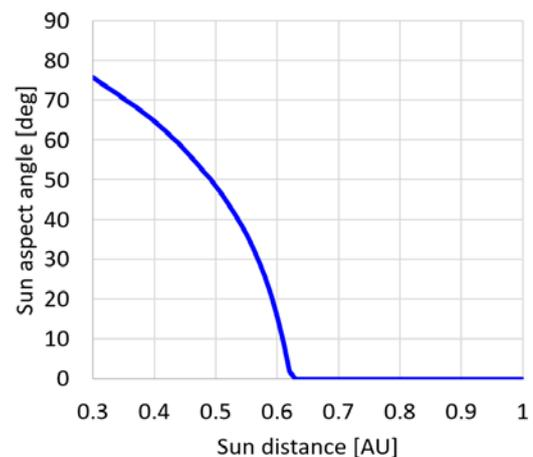
Figure 14: MTM solar array allowed Sun aspect angle depending on Sun distance (SAA of 0 deg means MTM SA is facing the Sun).
