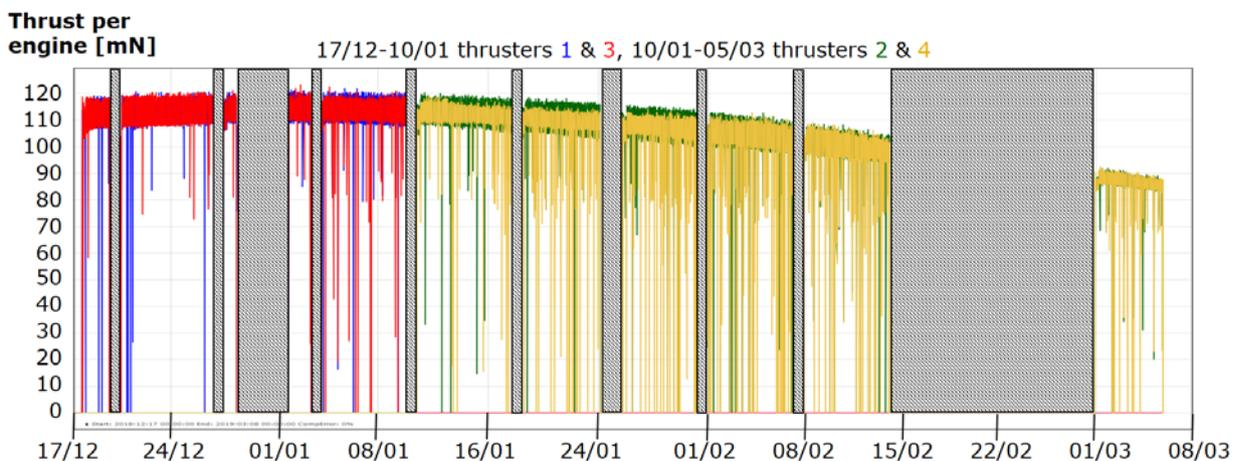
Figure 12: Thrusters and thrust levels used during the SEP1 arc. Greyed out periods indicate when the thrusters were OFF (S/C in NM). The large period before the last few days of thrusting in early March was to do an orbit determination with full accuracy prior to performing the final touch up manoeuvre of the arc.
