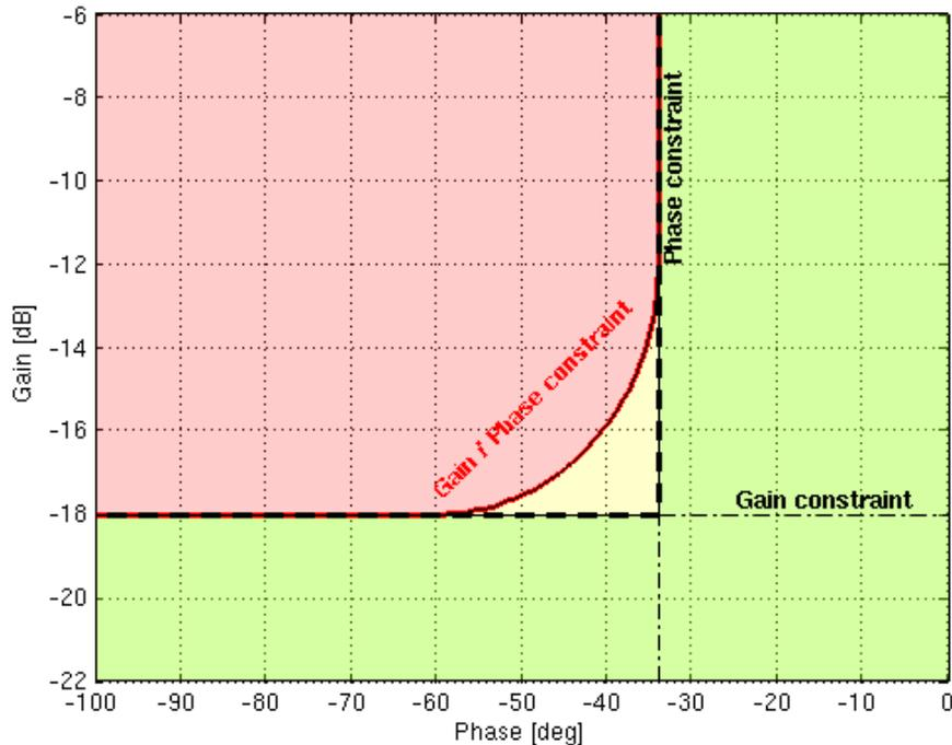
Figure 10: Gain and phase constraints at a given frequency
