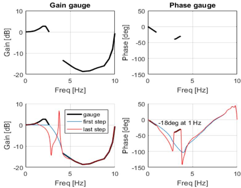
Figure 5: Gain attenuation and phase control with equivalent delay minimization
