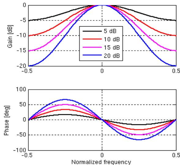
Figure 1: Cosine example Bode diagram
