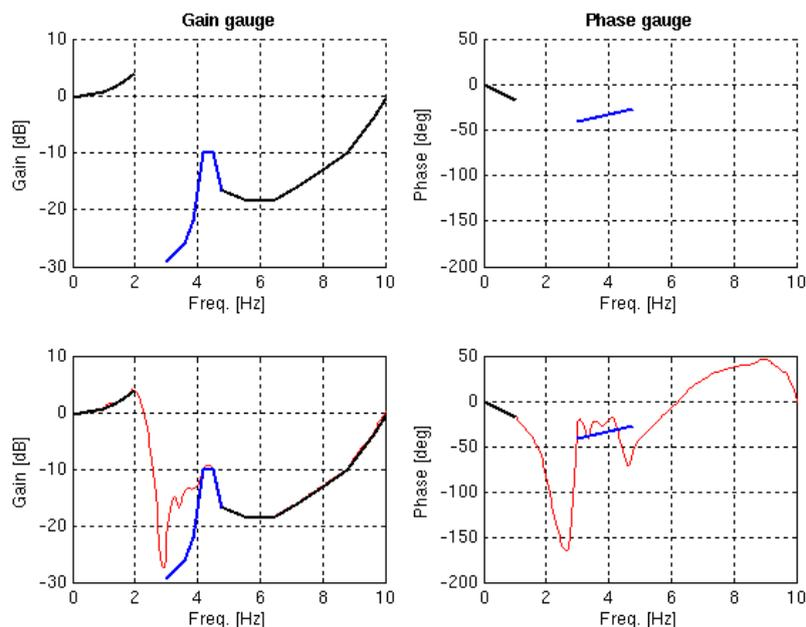
Figure 6: Mixed gain / phase control with equivalent delay minimization
