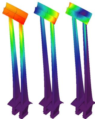
Figure 3: Modal shapes for welded in pairs configuration. Modes 1 to 3 from left to right.
