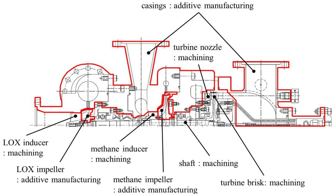
Figure 4: The manufacturing method of each part of the turbopump
