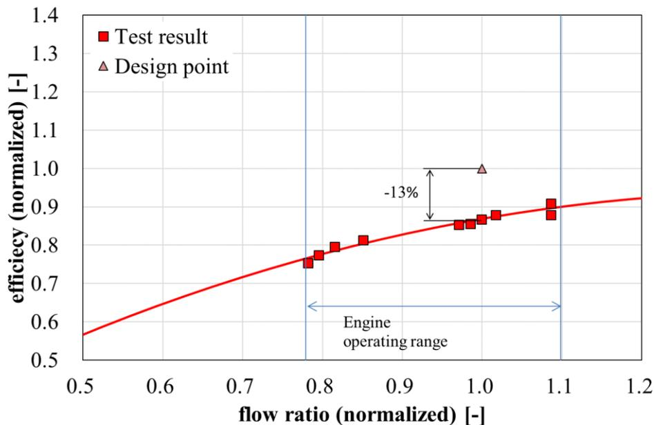
Figure 11: Efficiency of the methane pump (Vertical and horizontal axes normalized by design point)
