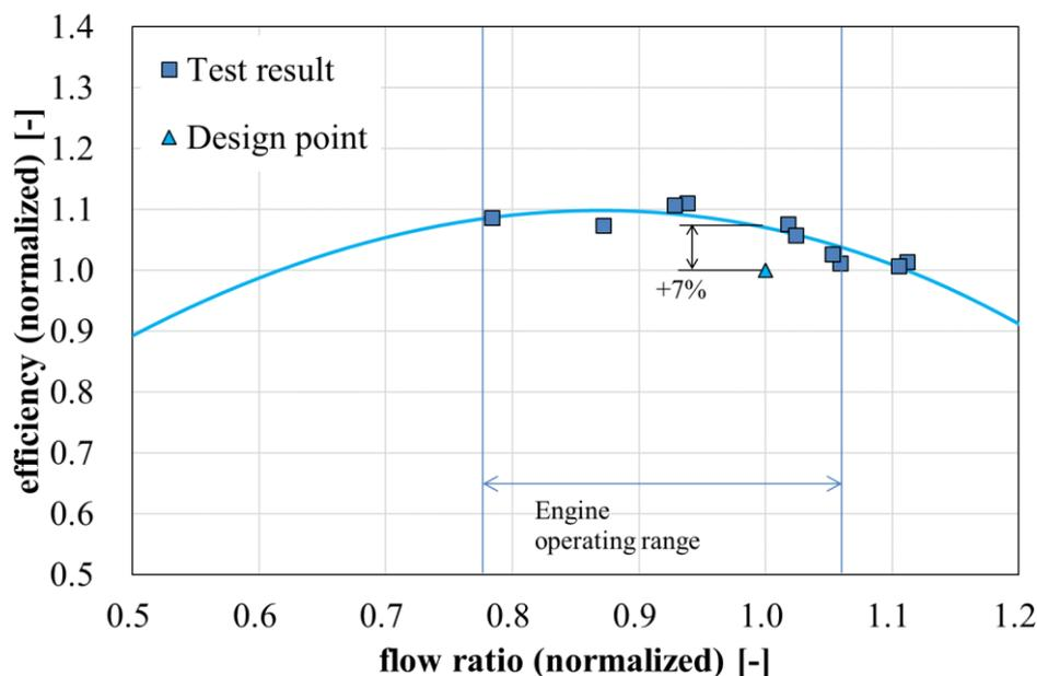
Figure 9: Efficiency of the LOX pump (Vertical and horizontal axes normalized by design point)
