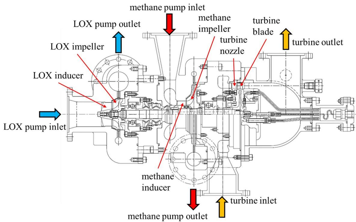
Figure 2: The half- sectional view of the turbopump
