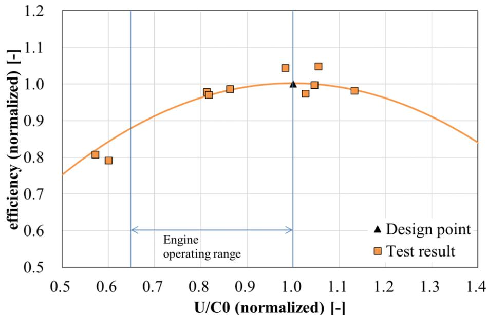
Figure 12: Efficiency of the turbine (Vertical and horizontal axes normalized by design point)
