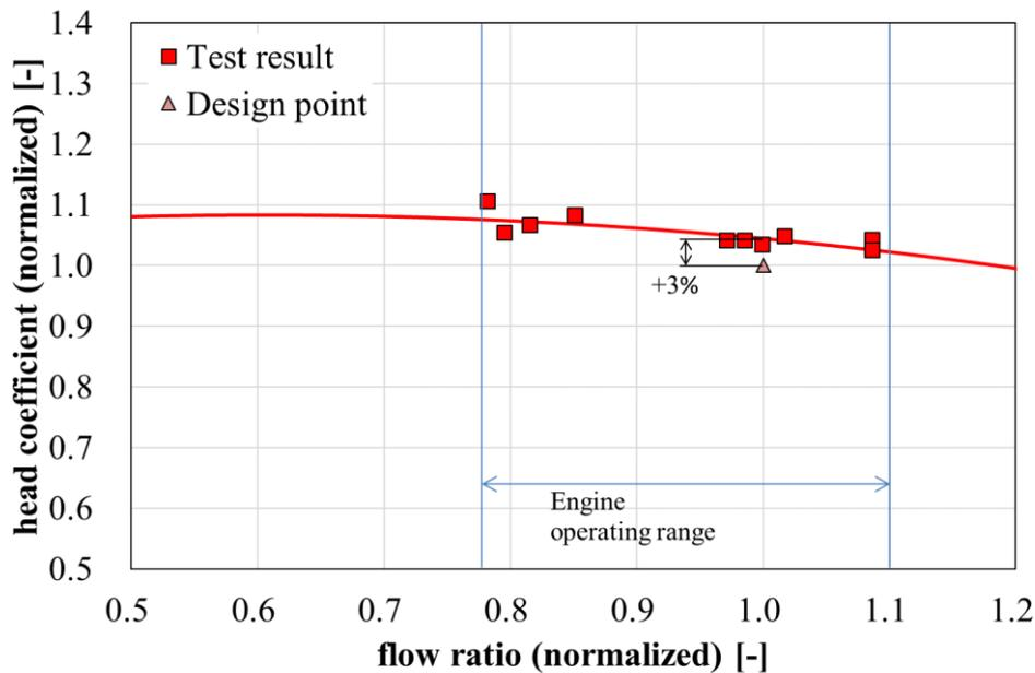
Figure 10: Head coefficient of the methane pump (Vertical and horizontal axes normalized by design point)
