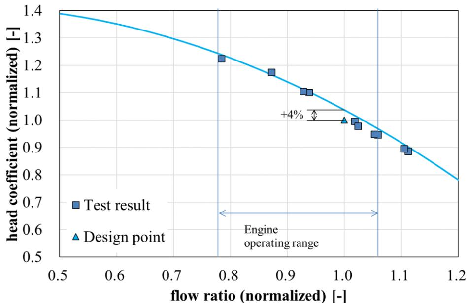
Figure 8: Head coefficient of the LOX pump (Vertical and horizontal axes normalized by design point)
