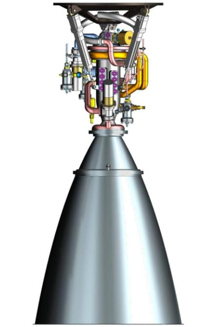
Figure 1: Schematic of full expander cycle engine
