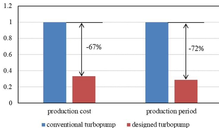
Figure 5: Comparison of production period and cost of the first prototype; the designed turbopump and the conventional turbopump
