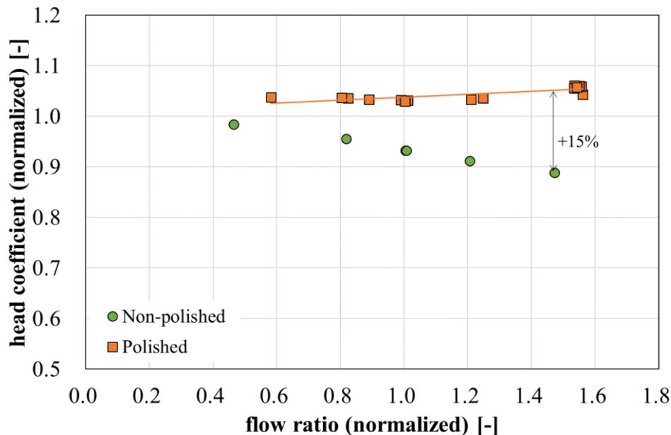
Figure 6: Comparison of head coefficient of impellers; additive manufacturing without polish and additive manufacturing with polish
