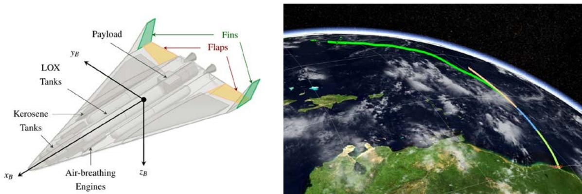
Figure 2: Overview of the reference concept Aurora-R2 and its optimized trajectory
