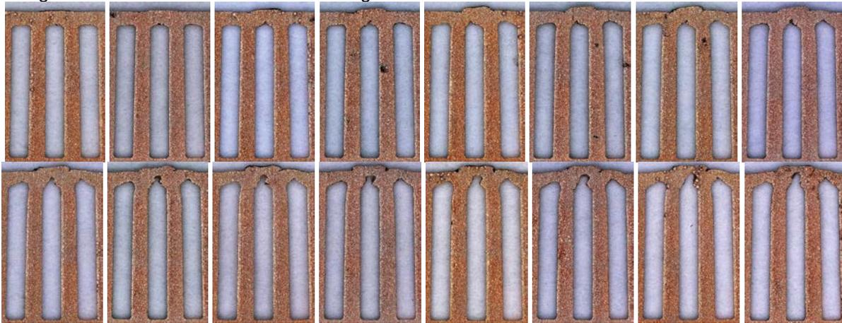
Figure 17: Cross sections of the AKIRA TMF panel (all at the failure cycle 369) in (from left to right and from top to bottom) decreasing distance to the crack.
