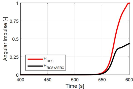
Figure 4: Impact on the resulting angular impulse required for RCS when using with and without aerodynamic controls
