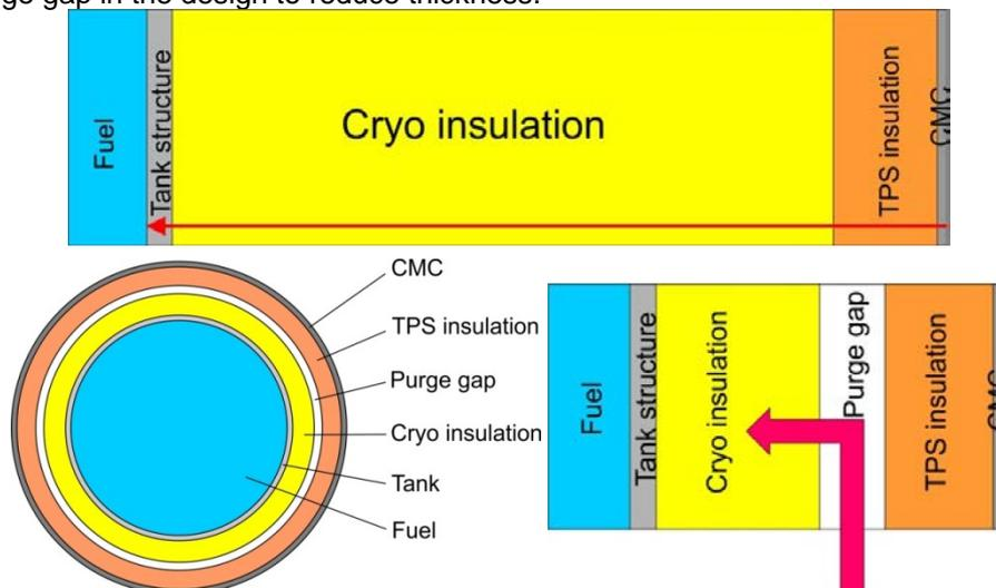
Figure 11: Schematics of conventional cryo-insulation combined with TPS (top) and alternative purge gap option (bottom) [21]
