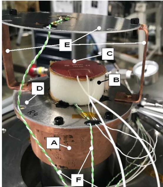
Figure 10: Complex test arrangement for determination of insulation foam heat conductivity (material probe is shown at B)
