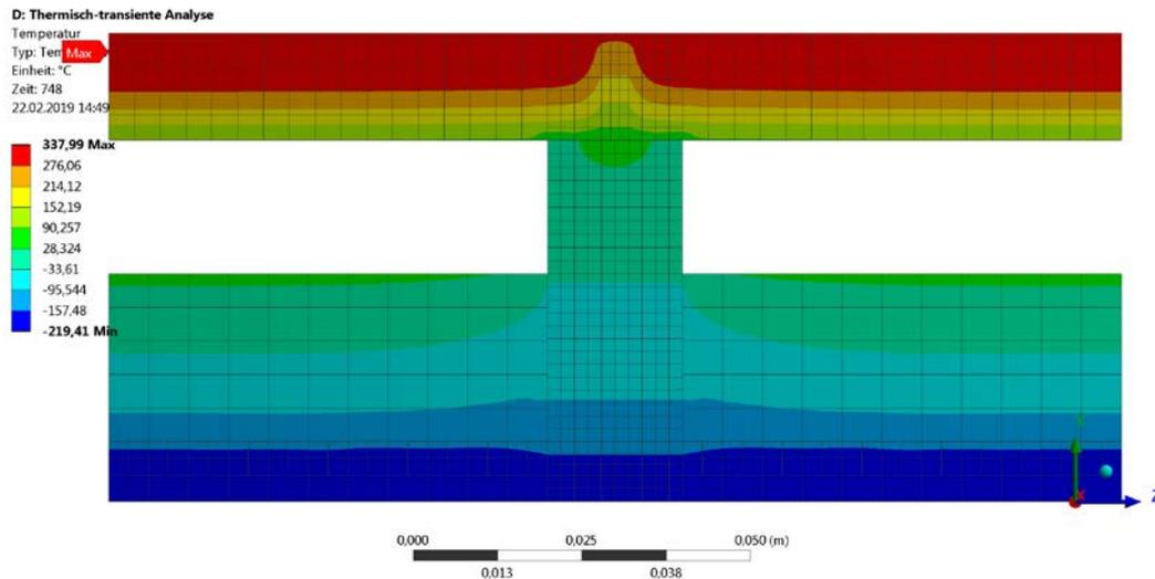
Figure 12: Transient simulation result at time when maximum temperature is reached on cryo-insulation (approx. 90°C below 100°C) [21]
