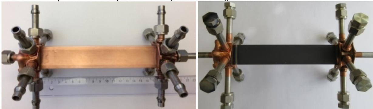
Figure 16: The AKIRA TMF panel made from CuCrZr in its laser-loading section (left) and coated AKIRA TMF panel (right)
