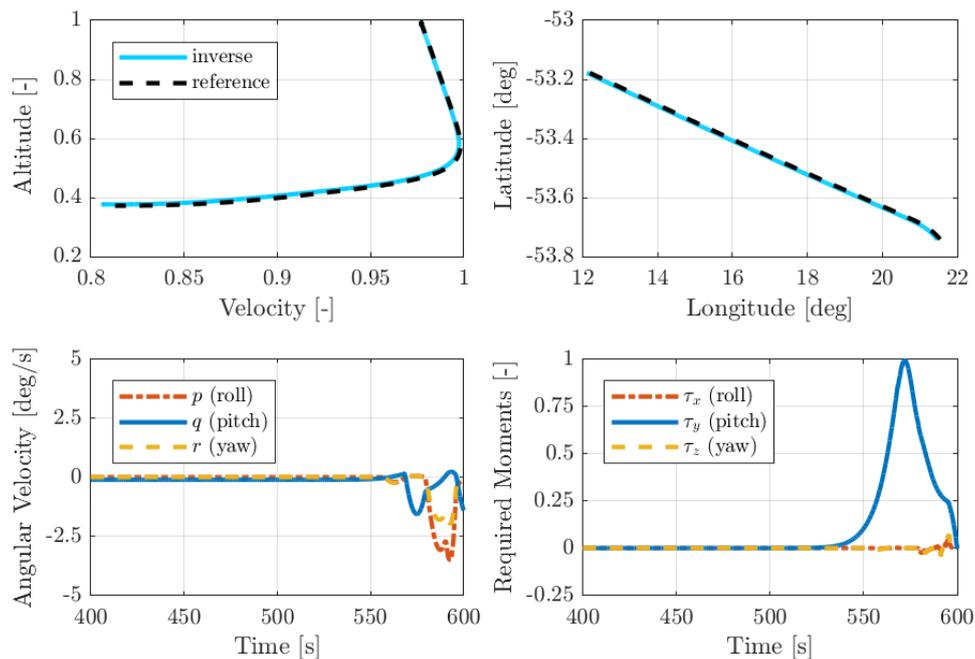
Figure 3: Aurora-R2 descent flight parameters obtained by nonlinear inverse modeling
