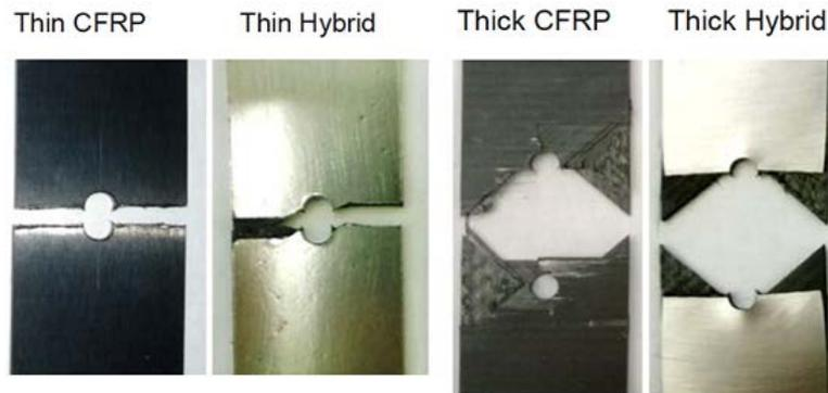
Figure 15: Different proof structures after Open-Hole-Tension tests
