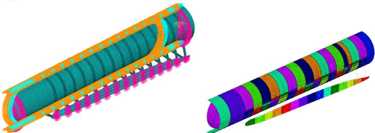
Figure 14: FEM model and constraints of RLV tank-wing intersection and HyperSizer components (right)
