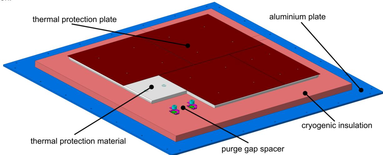
Figure 13: CAD Model of the largest Integrated Test Object (ITO) to be manufactured in AKIRA
