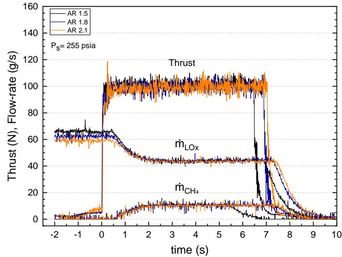
Fig. 4: Variation of thrust and propellant flow rate according to aspect ratio
