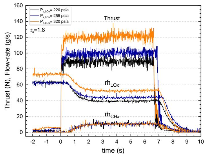
Fig. 3: Variation of thrust and propellant flow rate according to oxidizer supply pressure
