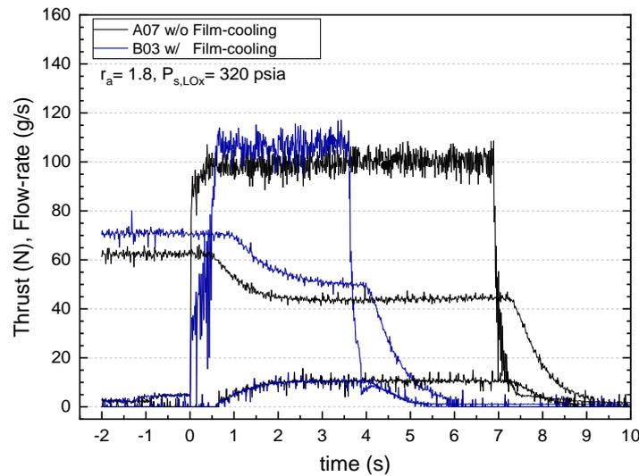
Fig. 6: Effects of film cooling on thrust performance
