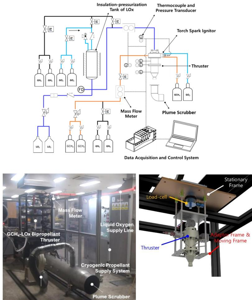
Fig. 1: Experimental setup
