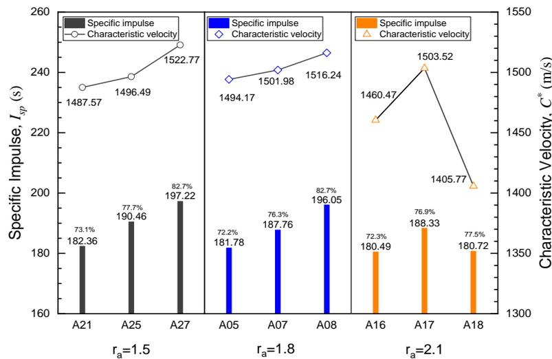
Fig. 5: Characteristic velocity and specific impulse with its efficiency
