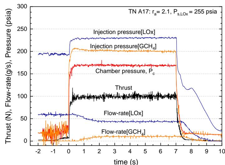
Fig. 2: Test result of case A17
