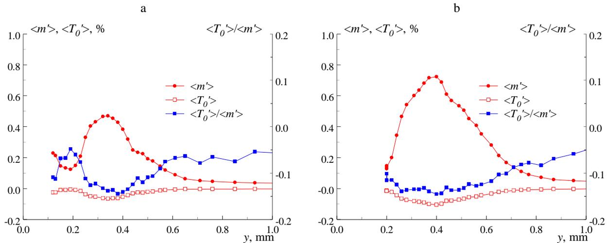
Figure 6: Profiles of Mass flow and total temperature pulsations at  $M_\infty=2$  (a) and  $M_\infty=2.5$ (b),  $Re_l \approx 11.4 \times 10^6 \text{ m}^{-1}$
