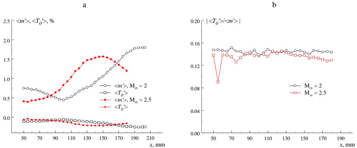
Figure 7: Development of boundary layer disturbances at  $Re_l = 11.4 \times 10^6 \text{ m}^{-1}$  and Mach numbers  $M_\infty = 2$  and  $M_\infty = 2.5$
