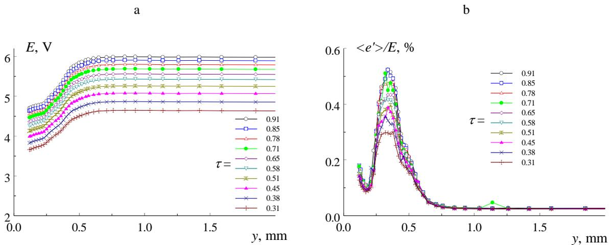
Figure 4: Profiles of mean voltage (a) and pulsating signal level (b) at various probe temperature load;  $x = 90$  mm,  $M_\infty = 2$ ,  $Re_l \approx 11.4 \times 10^6 \text{ m}^{-1}$
