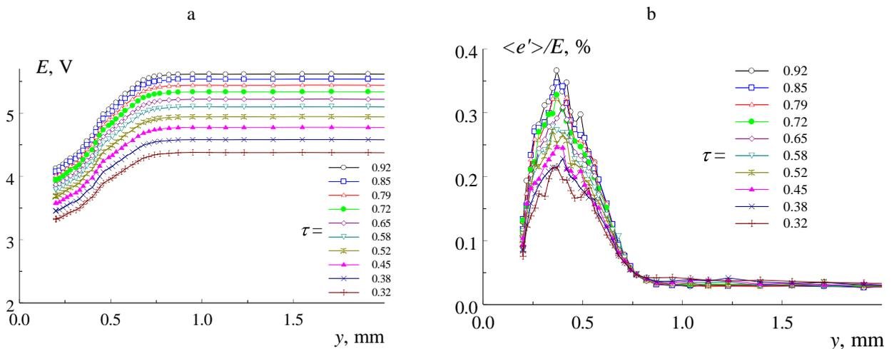
Figure 5: Profiles of mean voltage (a) and pulsating signal level (b) at various probe temperature load;  $x = 90$  mm,  $M_\infty = 2.5$ ,  $Re_l \approx 11.4 \times 10^6 \text{ m}^{-1}$
