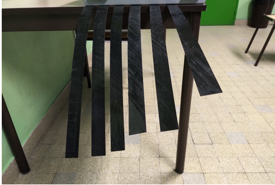
Figure 6: Laminate static deflection, from left to right : [90, 0, 90] , [60, 0, 60] , [45, 0, 45] , [30, -30, 30] , [30, 0, 30] and [15, 0, 15] .
