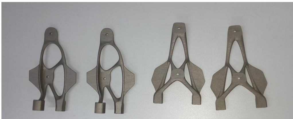
Figure 7: CHEOPS SA Brackets built with manufacturing aids for machining
