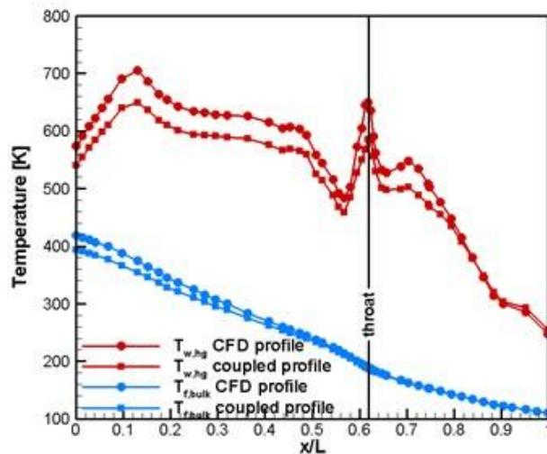
Figure 12: Cooling Jacket temperature axial profiles: wall temperature profile of the liner (red) and fluid bulk temperature (blue)
