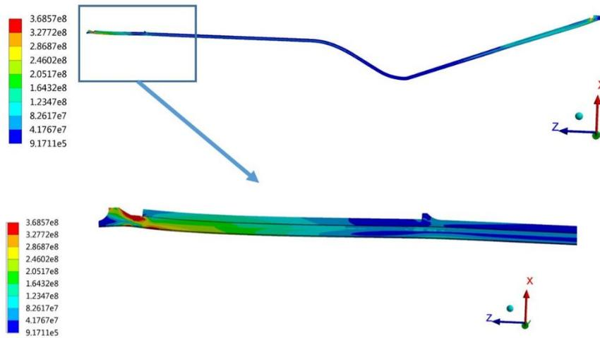
Figure 16: Von Mises Stresses (Pa) on the copper liner
