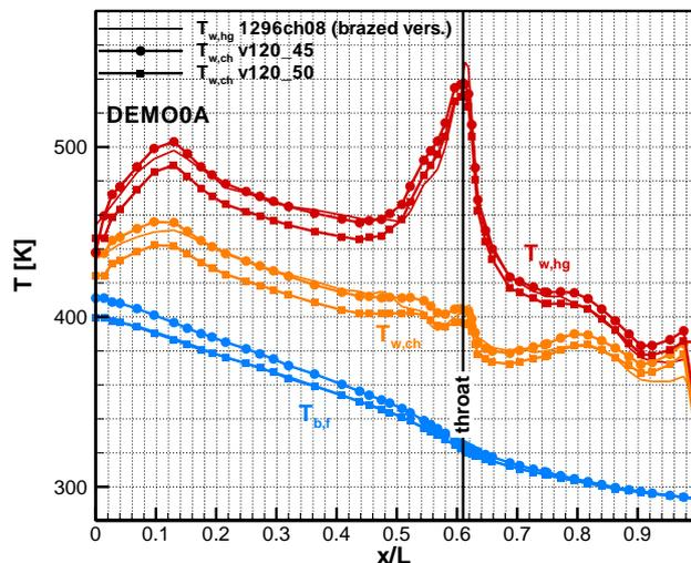
Figure 15: HYPROB DEMO cooling jacket: axial profiles for hot gas wall, channel bottom wall and fluid bulk temperature – “brazed” and “electroplated” versions
