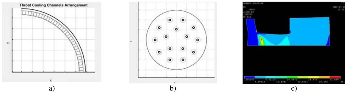
Figure 19: Throat channels arrangement, injectors' arrangement and Margin of Safety (MOS) in throat section
