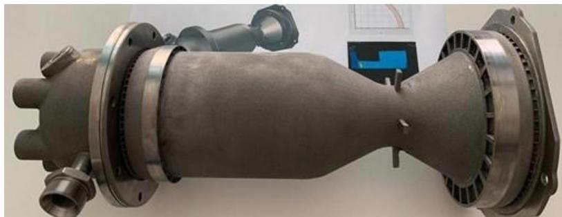
Figure 23: AM thrust chamber mock up printed and finished
