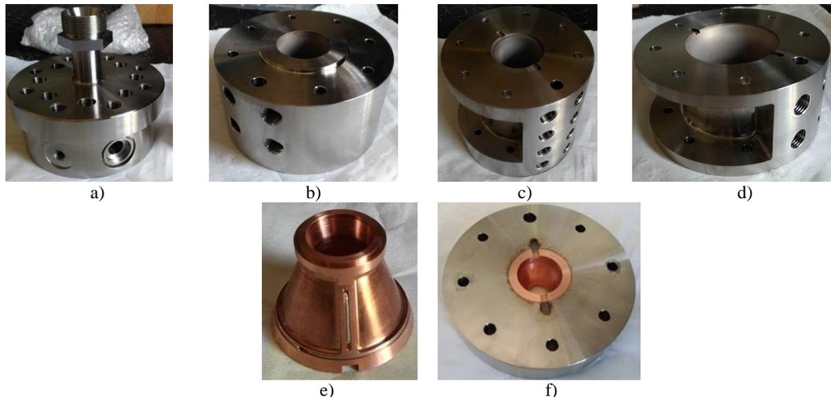
Figure 6: SSBB-CC modules in the manufacturing phase: a) injector plate; b) close-out of cylindrical part module 1; c) close-out of cylindrical part module 2; d) close-out of nozzle module; e) copper liner of throat module; f) assembly of throat module.
