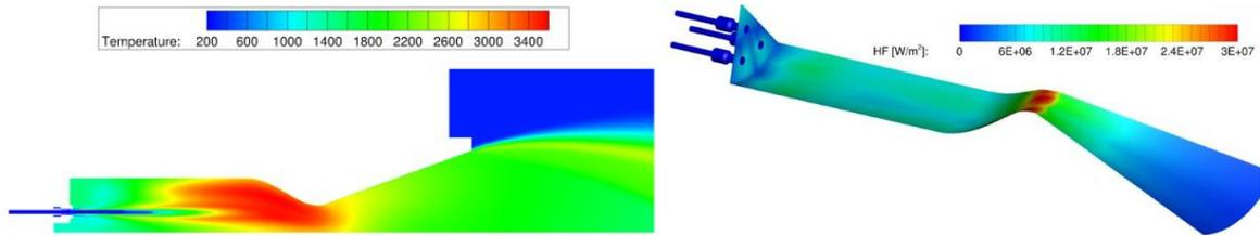
Figure 10: Temperature contour of FSBB combustion chamber and heat fluxes from 3D CFD dual step simulation
