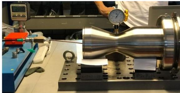
Figure 14: DEMO 1:1 mock up under proof test (up to 200bar)
