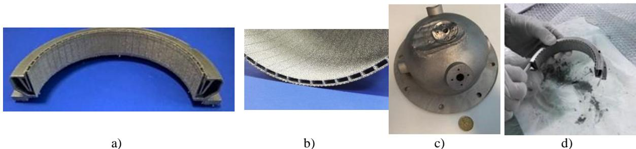
Figure 21: Printing experiments: manifold, combustion chamber, injector plate (erroneous supports design) ultrasonic cleaning
