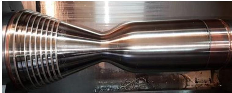
Figure 18: DEMO: Turning after nickel layer deposition
