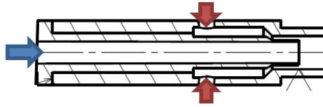
Figure 8: Sketch of the coaxial injector element (blue=oxygen, red=methane)
