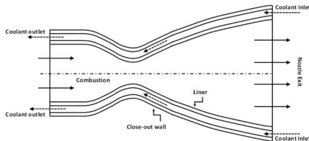
Figure 11: Counter-flow architecture of the cooling jacket
