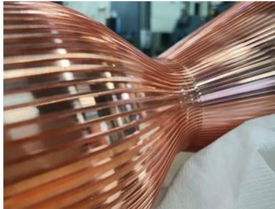
Figure 17: Details of the cooling channel after milling in the throat zone
