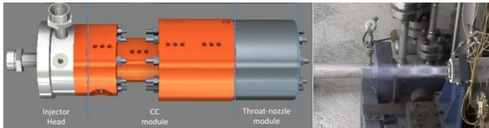
Figure 3: Test article detail and an image from test campaign
