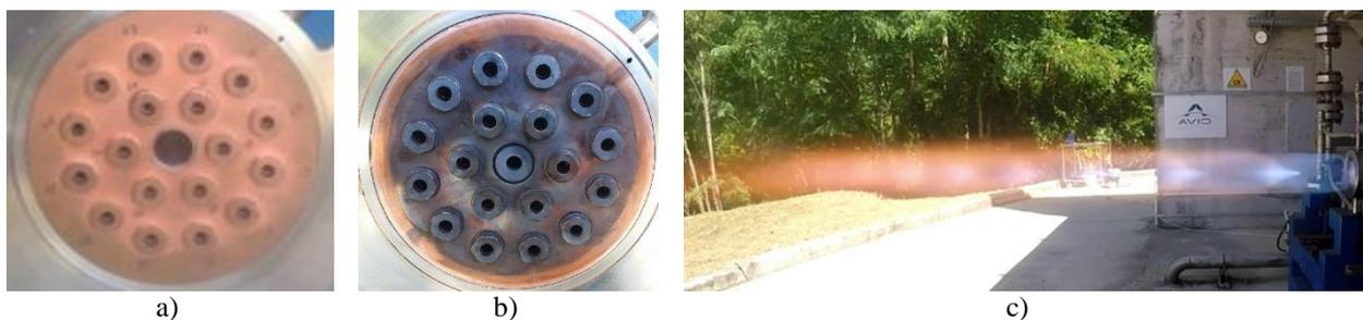
Figure 9: DEMO Injector head – Before (a) and after (b) test campaign. FSBB TCA a during firing test (c)
