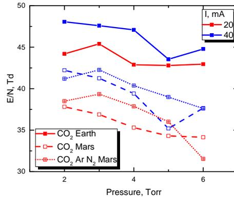
Figure 1: Measured variation of the reduced electric field as a function of the pressure at discharge currents 20 and 40 mA as a function of pressure for Earth-like temperature in pure  $\text{CO}_2$  and Mars-like temperature in pure  $\text{CO}_2$  and in mixture with argon and nitrogen.
