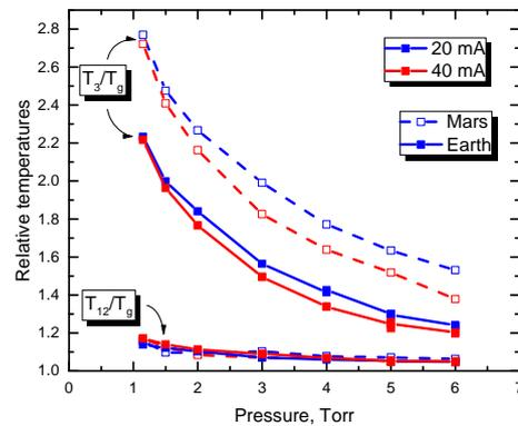
Figure 3: Relative temperatures measured as a function of a pressure at discharge current 20 and 40 mA at Mars and Earth temperature conditions.
