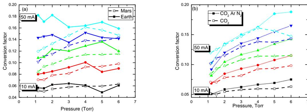
Figure 2: Measured conversion factor as function of pressure for different discharge currents, (—) 10 mA, (—) 20 mA, (—) 30 mA, (—) 40 mA, and (—) 50 mA: (a) for pure  $\text{CO}_2$  plasmas at Martian and Terrestrial temperature conditions; and (b) for pure  $\text{CO}_2$  and  $\text{CO}_2/\text{Ar}/\text{N}_2$  mixture at Martian temperature.
