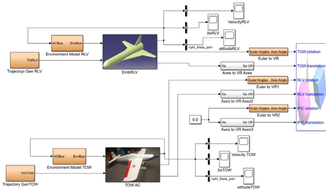
Figure 13: Simulink block diagram environment for multi-domain simulation
