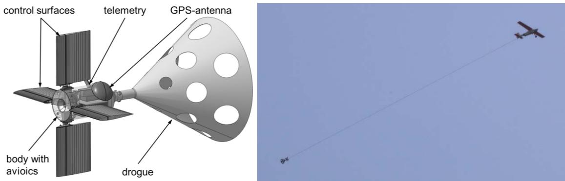
Figure 8: Coupling unit (left) and in flight test (right) with towing UAV "MAL" of DLR
