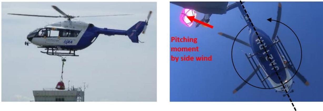
Figure 24: High-altitude drop test configuration and cause of the turn-over rotation just after the separation.
