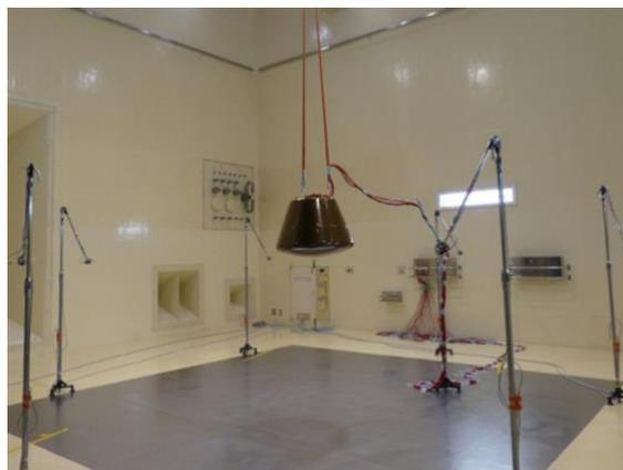
Figure 20: Acoustics vibration environmental test for the HSRC flight model.
