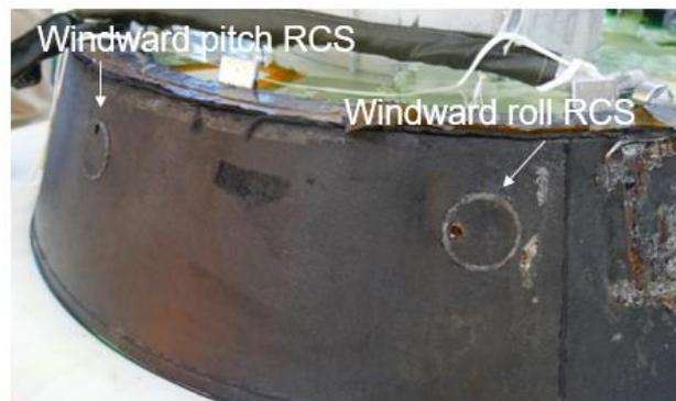
Figure 14: Windward ablator of the recovered HSRC.
