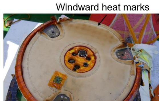
Figure 16: Hatch attachment side view of recovered HSRC.
