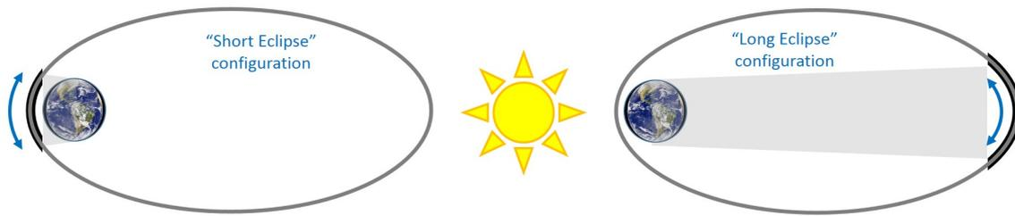
Figure 2: Different type of eclipses existing for high elliptically orbits
