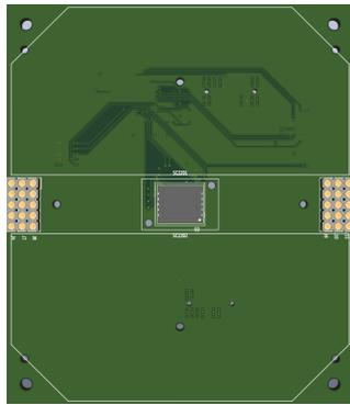
(a) Top view of the pogo pin interface on the HISP, with possible location of solar cells shown in the silkscreen.
