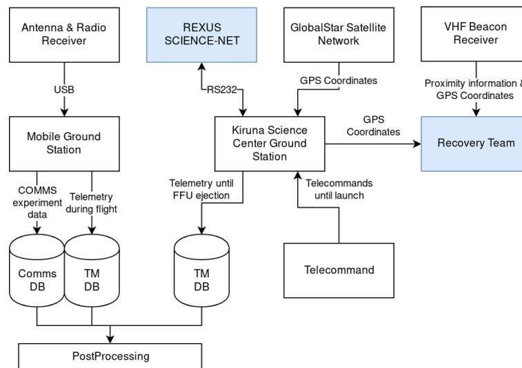
Figure 6: Overview of the components of the Ground Segment. Items in blue are provided by REXUS.
