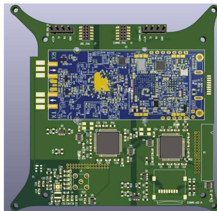
Figure 9: Front view of the PCDH PCB showing LimeSDR Mini<sup>27</sup> module.
