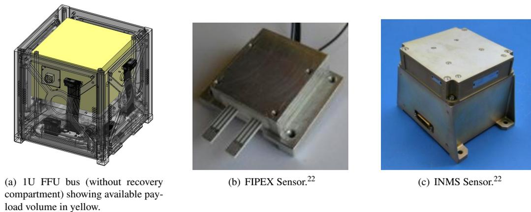
Figure 8: Payload volume in the TUPEX-7 FFU and possible future sensor payloads
