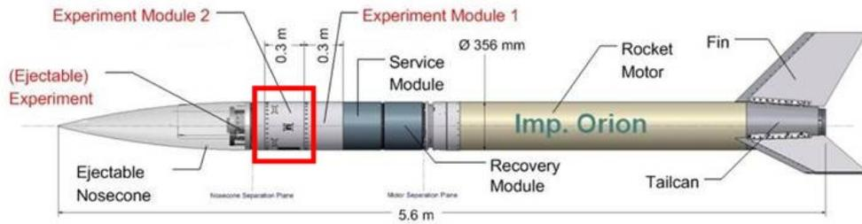
Figure 2: Representative image of the REXUS launch vehicle.<sup>15</sup> The location of the TUPEX-7 Experiment Module (next to the nosecone) is highlighted in red.
