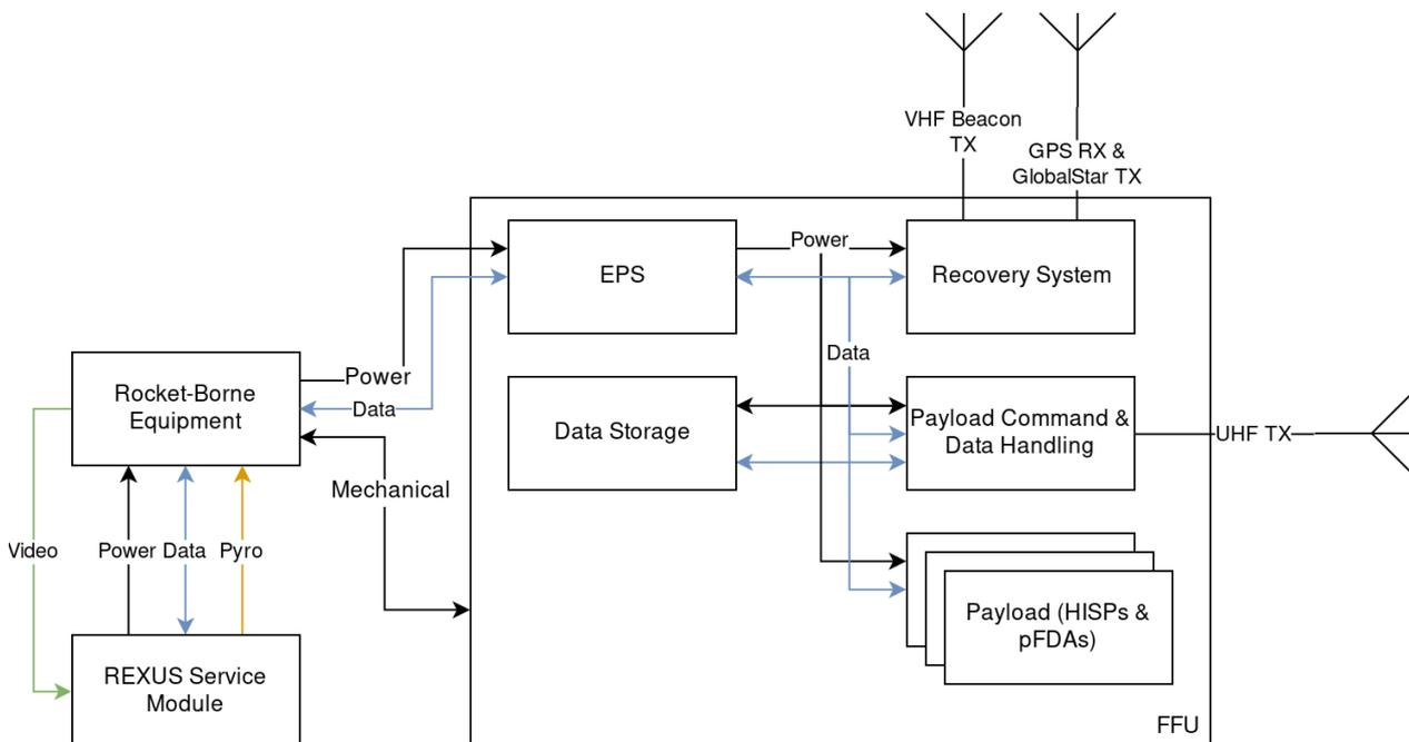
Figure 3: Schematic diagram of the components of the Space Segment.
