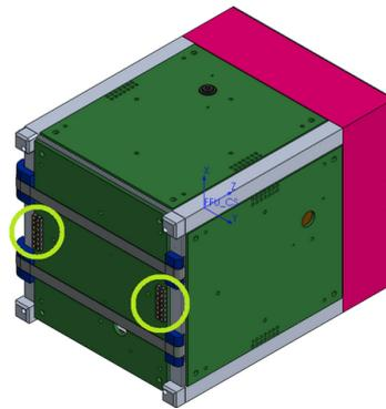
(b) Isometric view of the pogo pin target pads on the FFU
