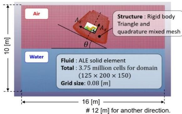
Figure 9: Computational grid for the water landing load analysis.
