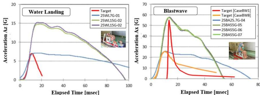
Figure 6: Hybrid III dummy sled test accelerations for the rigid seat [7].
