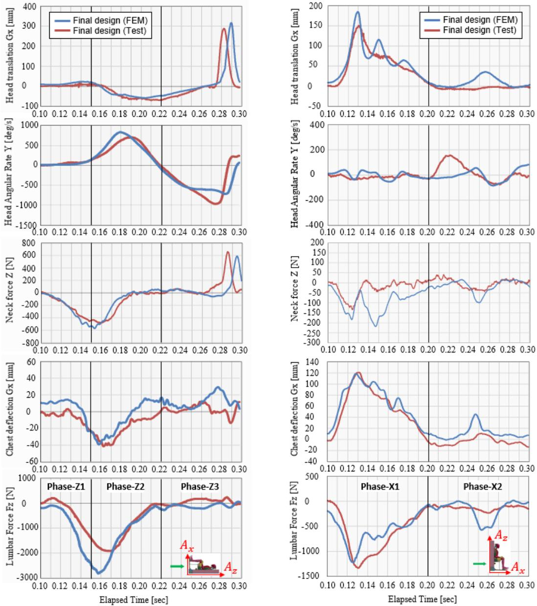
Figure 20: Hybrid III dynamic response for the final safety-designed spaceship seat DCSM-1401.
