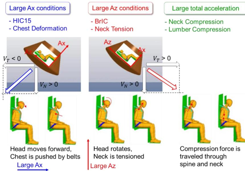
Figure 16: Crew injury biomechanics for the dynamic load due to excessive water landing velocity.
