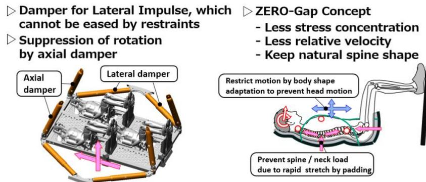
Figure 22: Proposed design-for-safety strategy to maximize the crew safety for the human space flight.
