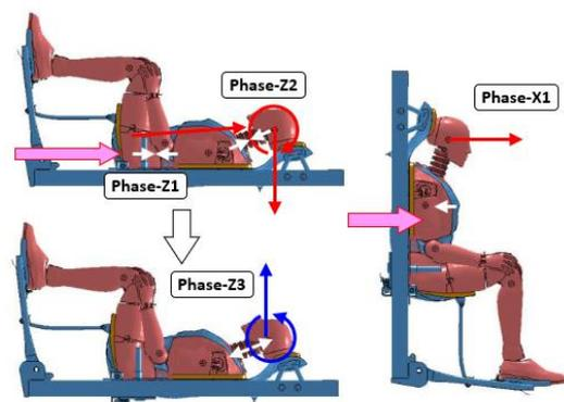
Figure 21: Dynamic behaviour of ATD for the design-for-safety seat.
