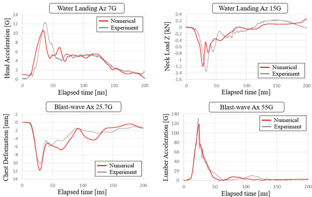
Figure 8: Comparisons of the experimental and predicted dynamic response of Hybrid III with the rigid seat [7].
