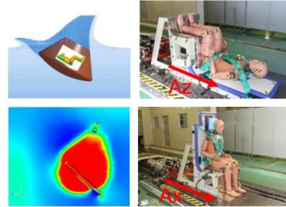
Figure 7: Hybrid III sled test configurations for the rigid seat.
