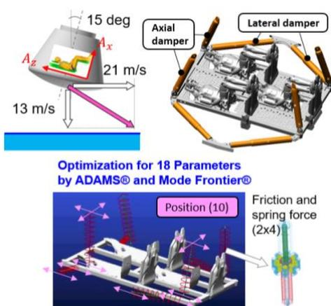
Figure 17: Design optimization for the spaceship dampers to reduce the acceleration level.
