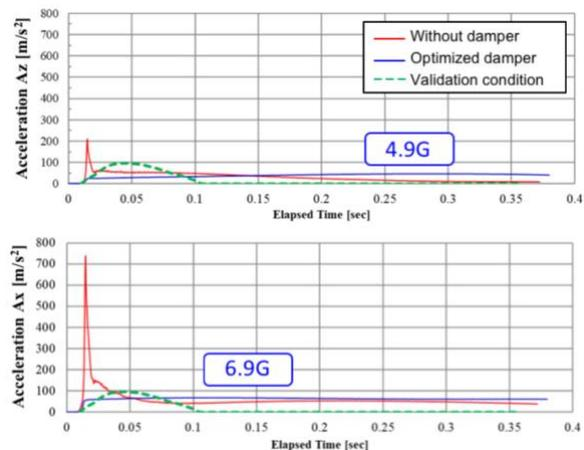
Figure 18: Design optimization result to reduce the acceleration level and the design validation condition.
