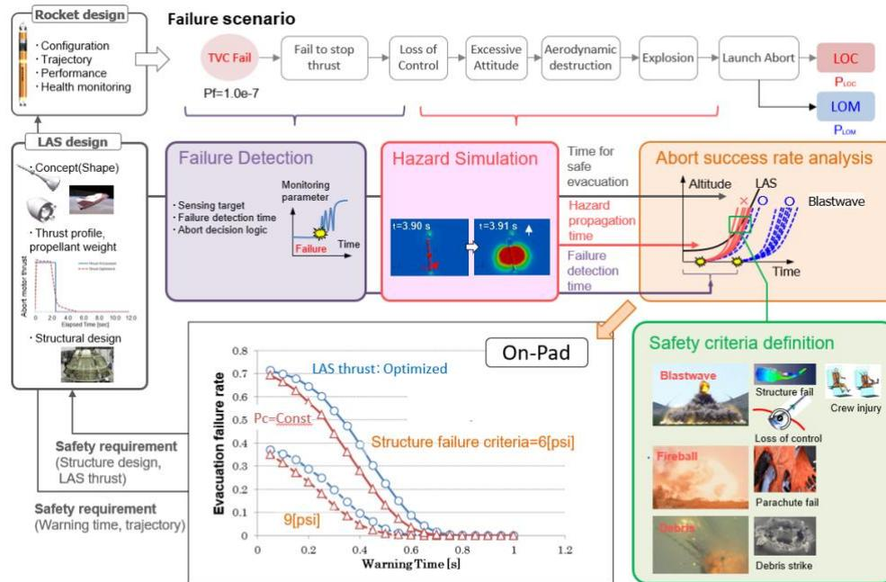
Figure 1: Quantitative crew safety analysis method for the evacuation success rate of LAS [2].
