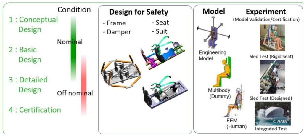
Figure 24: Design for safety process based on quantitative safety assessment for spaceship seats.
