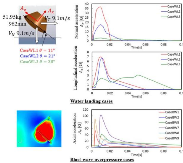
Figure 5: Dynamic accelerations for the water landing and the blast-wave overpressure [19].
