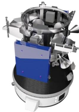
Figure 4: AOM with SAW in stowed configuration
