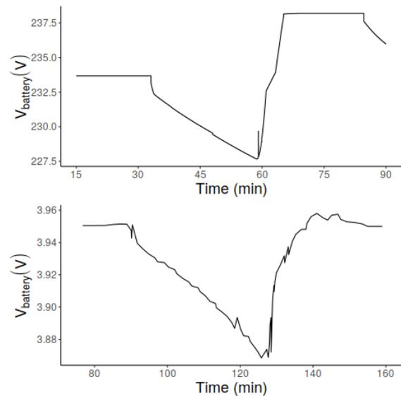
Figure 9: Battery voltage in simulation (top) and in reference data<sup>5</sup> (bottom)
