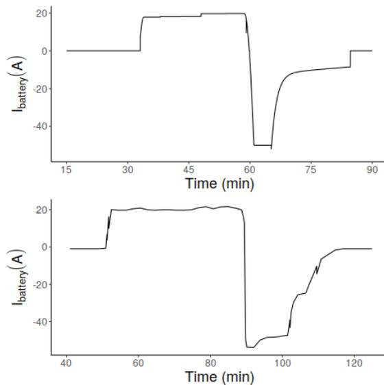
Figure 8: Battery current in simulation (top) and in reference data<sup>5</sup> (bottom).
