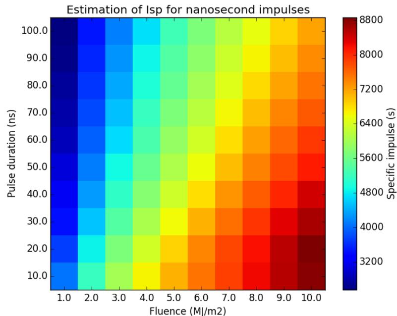
Figure 3 : Isp estimation using ESTHER for a fluence range from 1 to 10 MJ/m<sup>2</sup>, and a pulse duration from 10 to 100 ns
