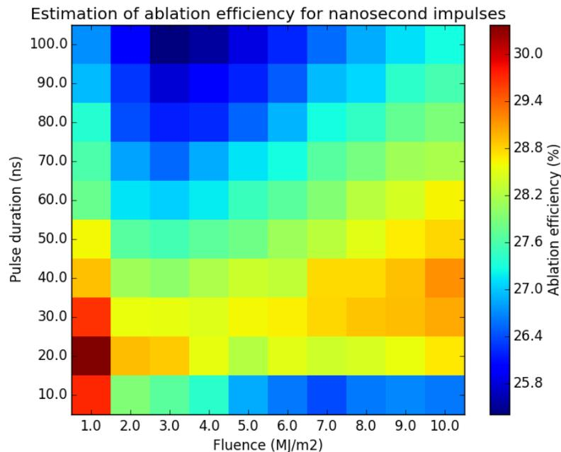
Figure 4 : Ablation efficiency estimation using ESTHER for a fluence range from 1 to 10 MJ/m<sup>2</sup>, and a pulse duration from 10 to 100 ns
