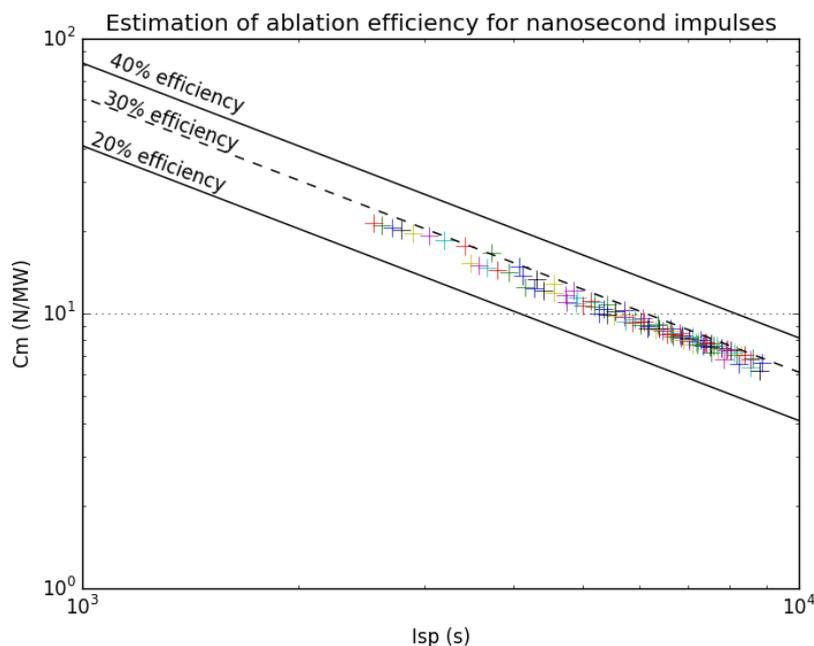
Figure 5:  $I_{sp}$  vs.  $C_m$  for every case computed, comparison with iso-efficiency lines.
