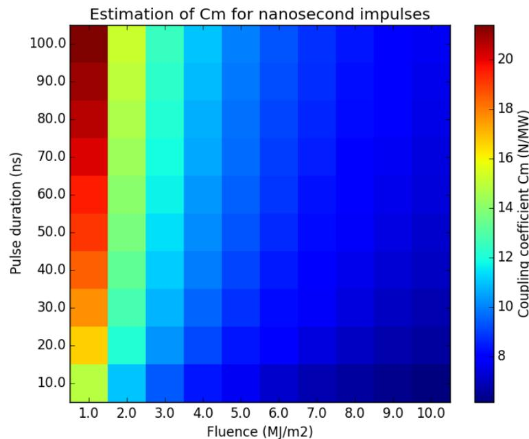
Figure 2 : Cm estimation using ESTHER for a fluence range from 1 to 10 MJ/m<sup>2</sup>, and a pulse duration from 10 to 100 ns
