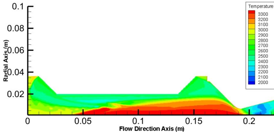
Figure 4: Static Temperature Distribution in SRM
