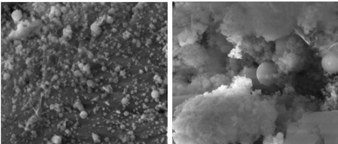
Figure 15: Al Particles under SEM
