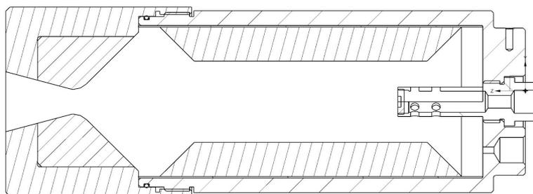
Figure 8: Small Scale Test Motor
