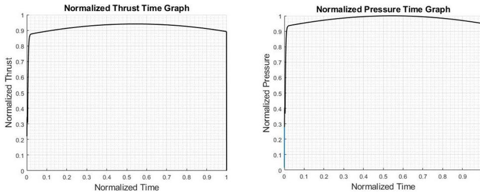
Figure 9: Small Scale Test Motor Normalized Thrust and Pressure History
