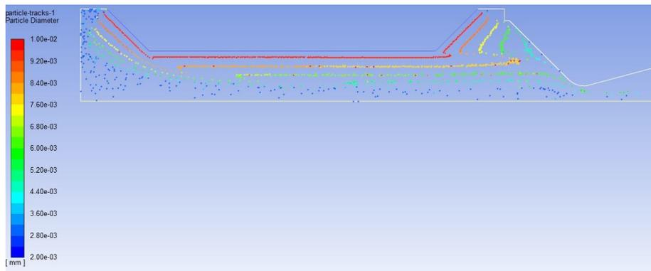
Figure 7: Particle trajectories inside SRM
