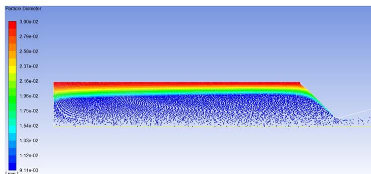
Figure 3: Particle Trajectory and Particle Diameter
